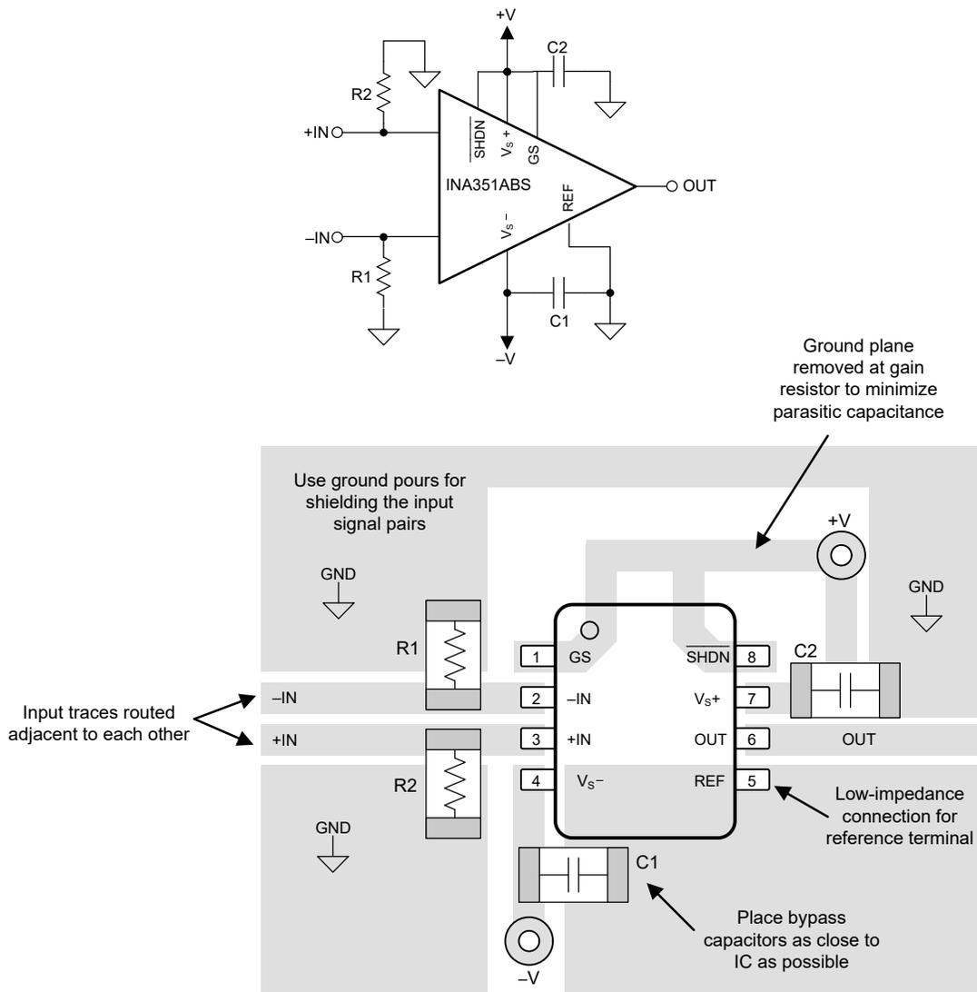
図 8-7. Example Schematic and Associated PCB Layout
