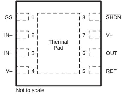
Note: Connect Thermal Pad to (V-)
