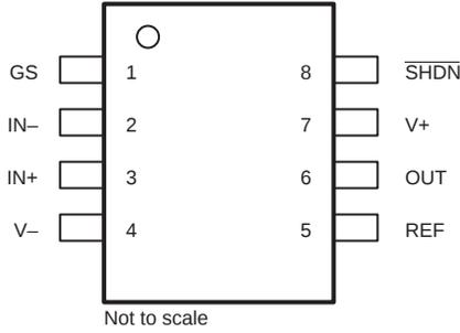
☒ 5-1. DDF Package, 8-Pin SOT-23 (Top View)
