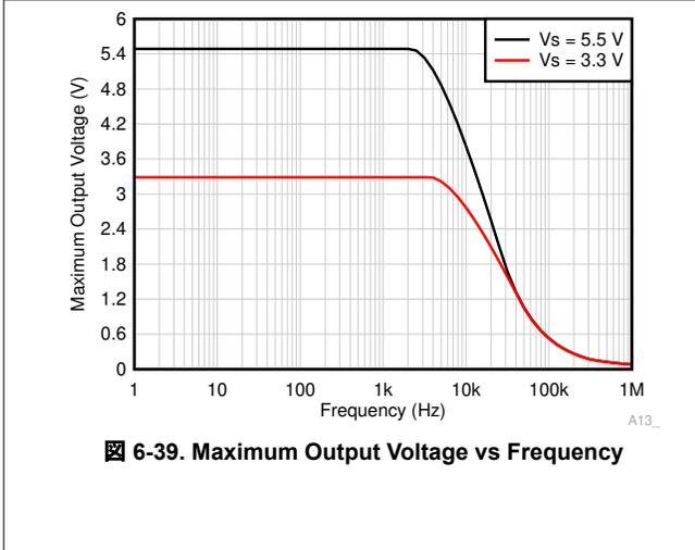
Figure 6-39. Maximum Output Voltage vs Frequency
