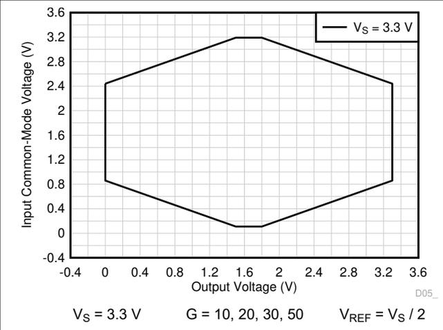
6-62. Input Common-Mode Voltage vs Output Voltage
