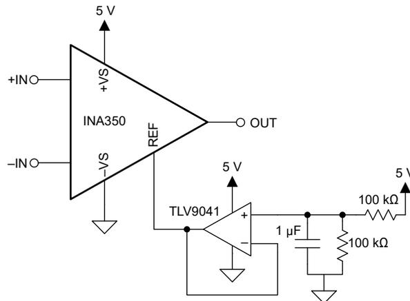
**Figure 8-1. INA350 / Traditional INA – External Reference Buffer Required**
