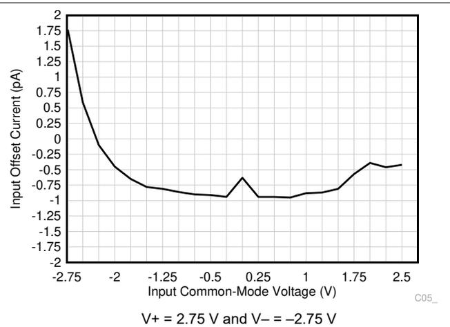
6-26. Input Offset Current vs Input Common-Mode Voltage
