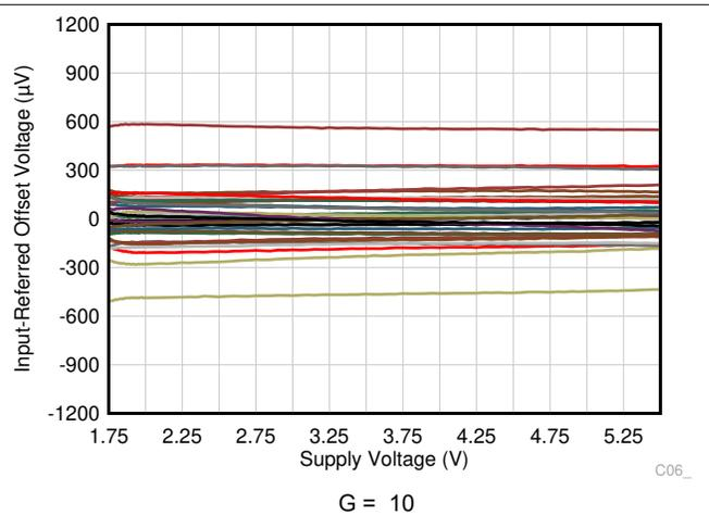
6-28. Input Referred Offset Voltage vs Supply Voltage
