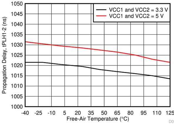
**6-10. t<sub>PLH1-2</sub> Propagation Delay vs Free-Air Temperature**
