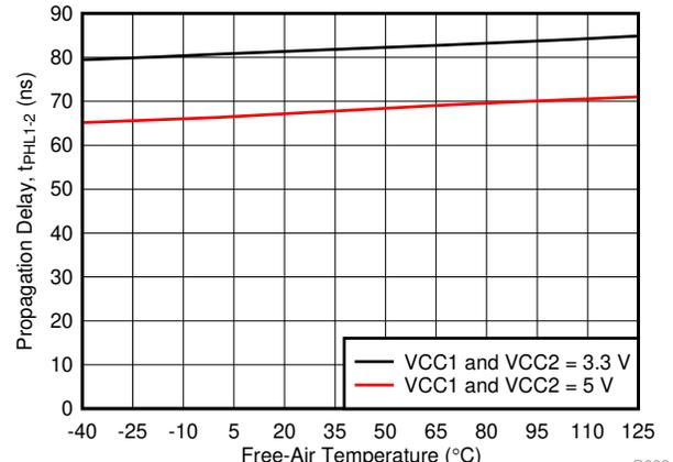
**6-11. t<sub>PHL1-2</sub> Propagation Delay vs Free-Air Temperature**
