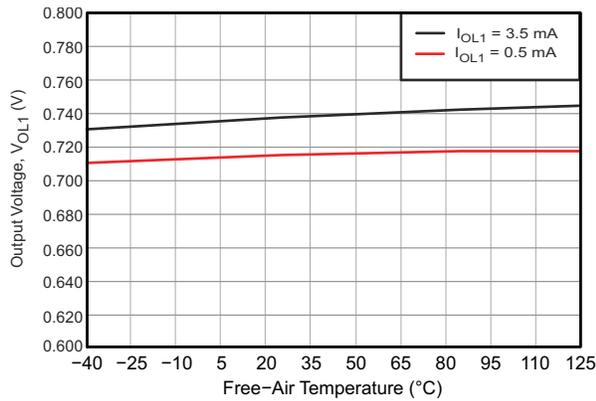
**6-2. Side 1: Output Low Voltage vs Free-Air Temperature**
