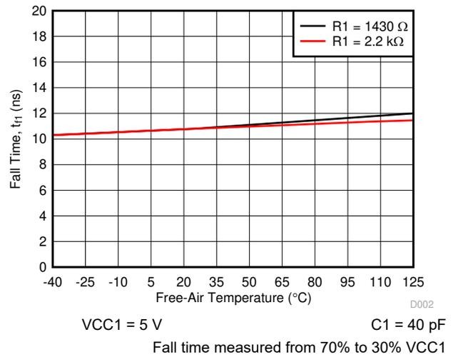
**6-5. Side 1: Output Fall Time vs Free-air Temperature**
