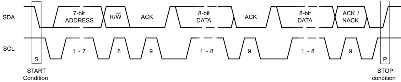
8-2. Timing Diagram of a Complete Data Transfer
