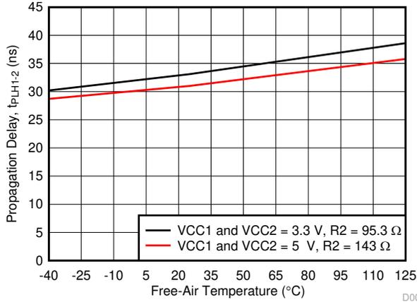
**6-8. t<sub>PLH1-2</sub> Propagation Delay vs Free-Air Temperature**
