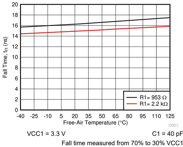
**6-4. Side 1: Output Fall Time vs Free-Air Temperature**
