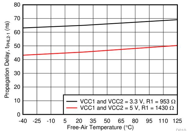
**6-13. t<sub>PHL2-1</sub> Propagation Delay vs Free-Air Temperature**
