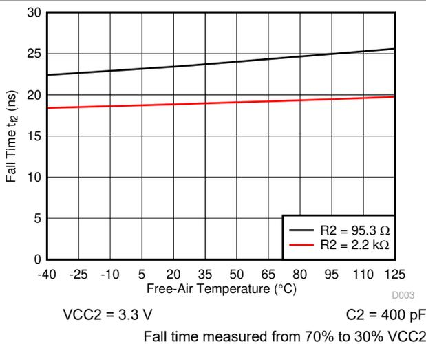
**6-6. Side 2: Output Fall Time vs Free-Air Temperature**
