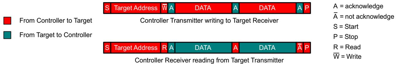
8-3. Transmit or Receive Mode Changes During a Data Transfer
