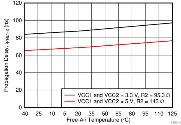
**6-9. t<sub>PHL1-2</sub> Propagation Delay vs Free-Air Temperature**
