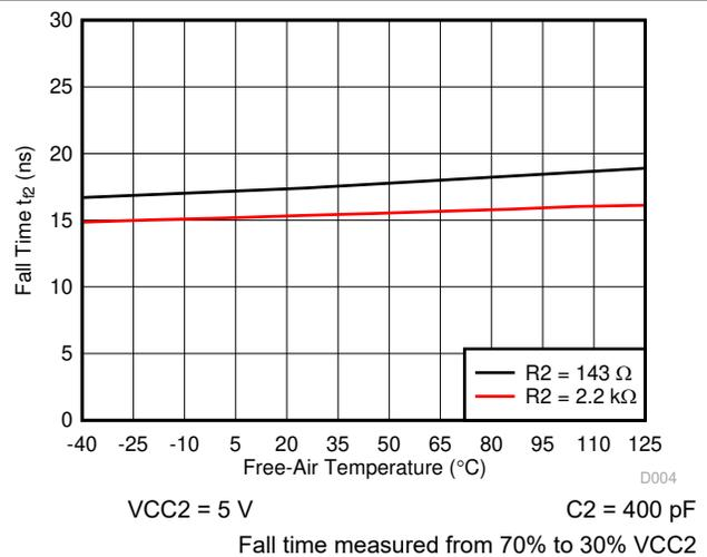
**6-7. Side 2: Output Fall Time vs Free-Air Temperature**
