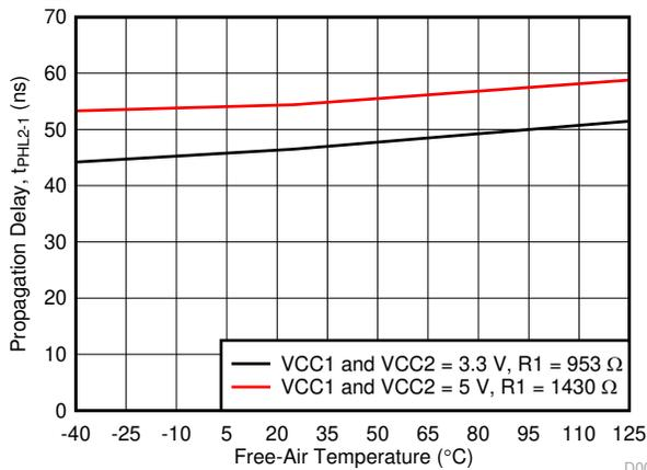
**6-12. t<sub>PHL2-1</sub> Propagation Delay vs Free-Air Temperature**
