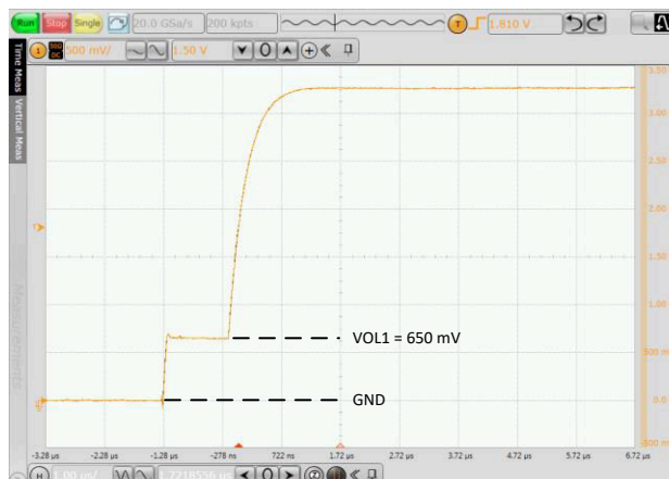
Figure 9-8. Side 1 ISO1640: Low-to-High Transition
