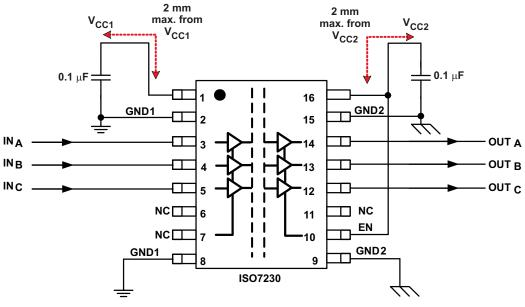
Figure 13. Typical ISO7230 Application Circuit
