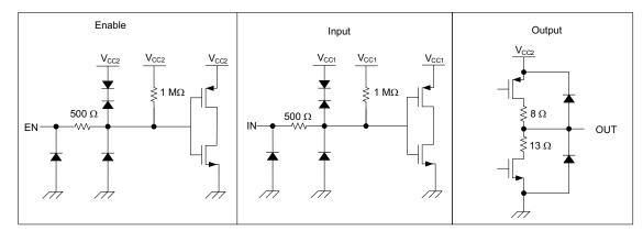
NOTE: Input is assumed to be on  $V_{\text{CC1}}$  side and Output on  $V_{\text{CC2}}$  side.
