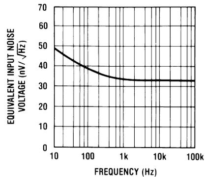
18. Equivalent Input Noise Voltage
