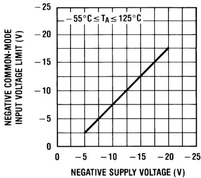
5. Negative Common-Mode Input Voltage Limit
