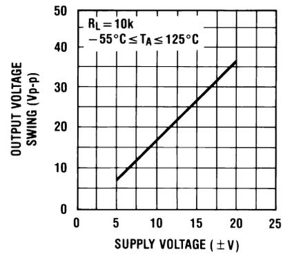
Fig 8. Output Voltage Swing
