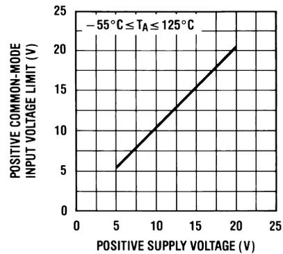
4. Positive Common-Mode Input Voltage Limit
