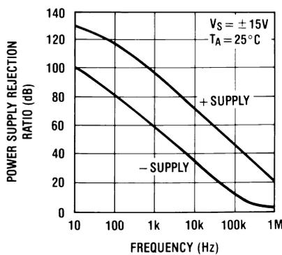
17. Power Supply Rejection Ratio
