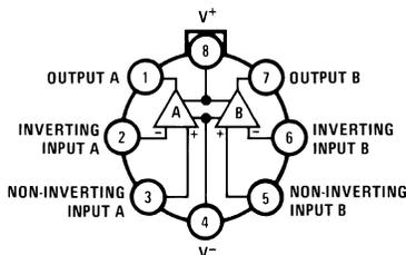
Pin 4 connected to case
