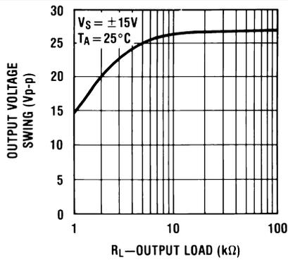
Fig 9. Output Voltage Swing
