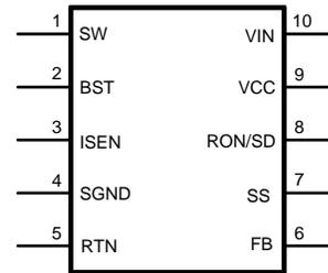
**Figure 2. 10-Lead WSON (Top View)**
