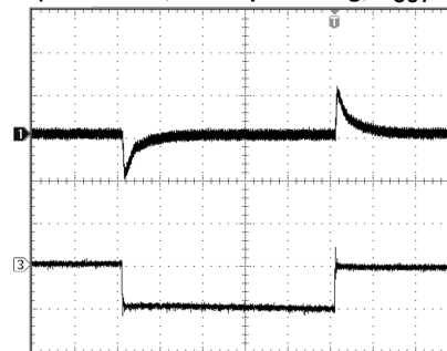
Line Step (LED Mode) (2 x 5 LEDs, 30mA per String, C_{OUT} = 1\mu F )
