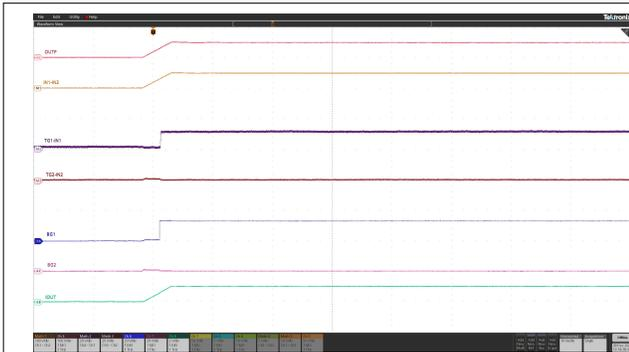
8-2. +48V DC Input, Startup with Vin Ramp
