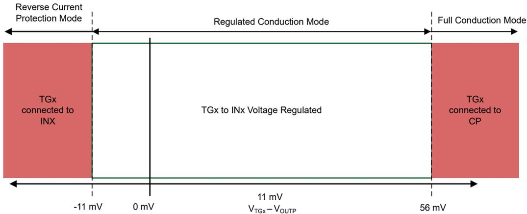
depicts how the modes of operation vary according to the DRAIN to SOURCE voltage. The threshold between forward regulation and conduction modes is when the DRAIN to SOURCE voltage is  $V_{TG\_REG}$ . The threshold between forward regulation mode and reverse current protection mode is when the DRAIN to SOURCE voltage is  $V_{REV}$ .
