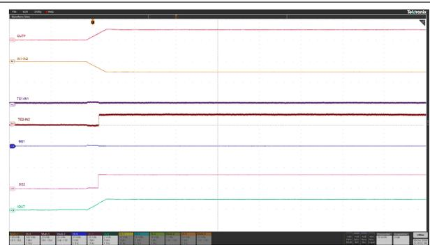
8-3. -48V DC Input, Startup with Vin Ramp
