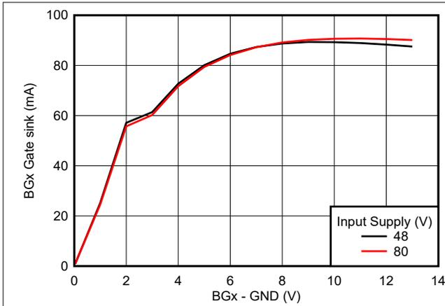
Figure 5-7. Bottom Side Gate Drive Sink Current vs Gate Drive Voltage
