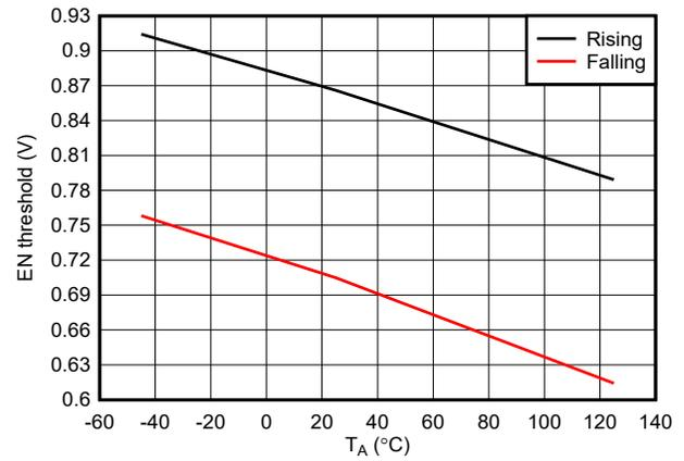
Figure 5-8. Enable Threshold vs Temperature
