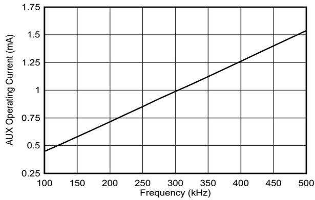
图 5-3. AUX Operating Current vs Frequency
