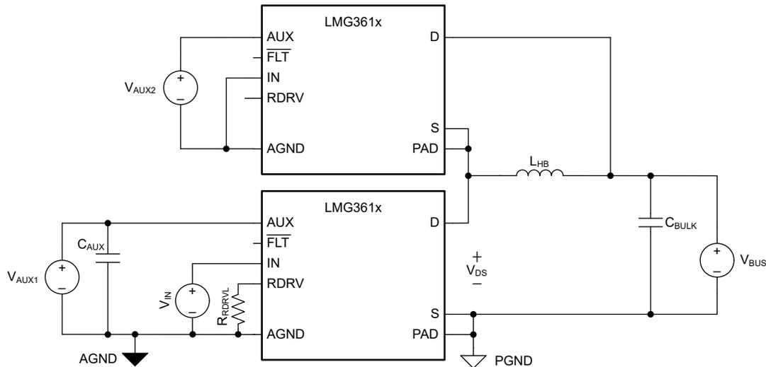
6-1. GaN Power FET Switching Parameters Test Circuit
