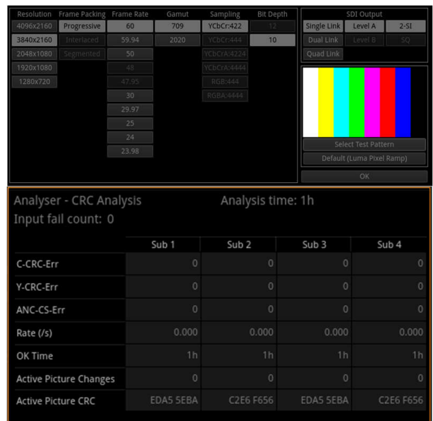
図 7-10. OUT0± BER at 11.88Gbps (12G-SDI), CC = 100m Belden 1694A, Reclocked
