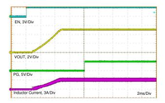
$\boxtimes$  8-4. Typical Start-Up Behavior  $V_{IN}$  = 12 V,  $V_{OUT}$  = 5 V,  $I_{OUT}$  = 3 A
