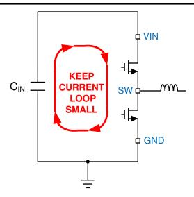
図 11-1. Current Loops with Fast Edges
