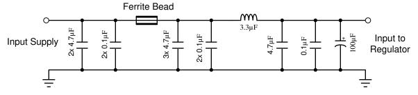
図 9-28. Typical Input EMI Filter
