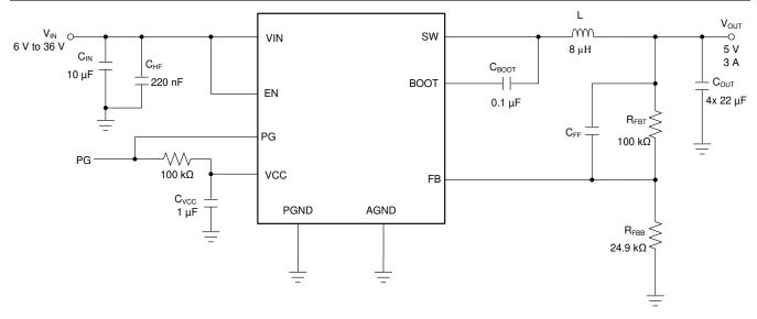
図 9-1. Example Application Circuit (400 kHz)
