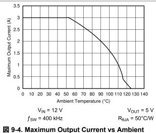
図 9-4. Maximum Output Current vs Ambient Temperature
