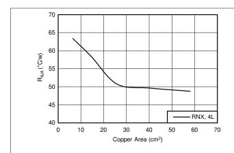
図 9-3. R<sub>θJA</sub> vs Copper Board Area for the VQFN (RNX) Package
