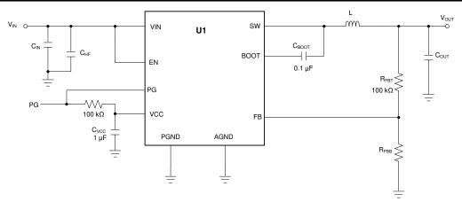
図 9-27. Circuit for Application Curves
