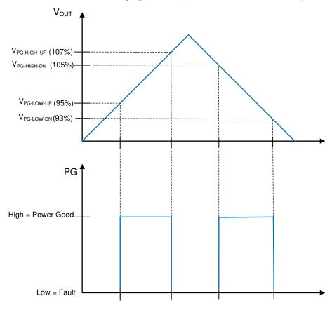
図 8-1. Static Power-Good Operation
