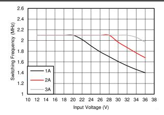
$\boxtimes$  8-13. Switching Frequency vs Input Voltage  $V_{OUT}$  = 3.3 V
