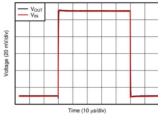
$G = 1$ ,  $V_{IN} = 100\text{mV}_{PP}$ ,  $C_L = 10\text{pF}$
