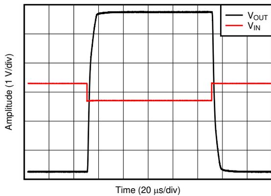
$G = -10$ ,  $V_{IN} = 600\text{mV}_{PP}$
