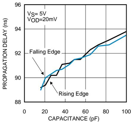
Figure 11. Propagation Delay vs. Capacitive Load
