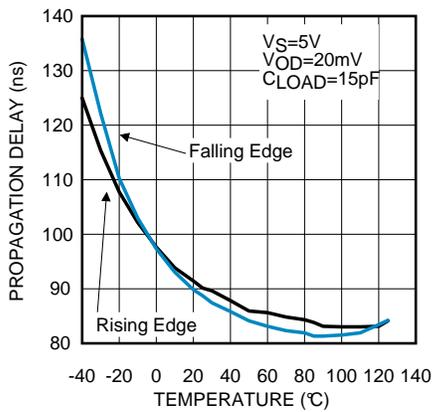
Figure 9. Propagation Delay vs. Temperature
