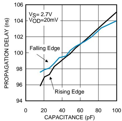
Figure 10. Propagation Delay vs. Capacitive Load
