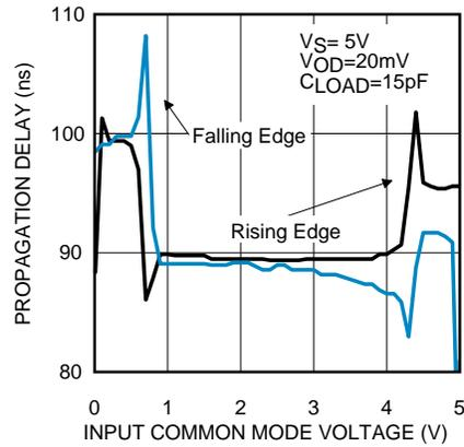
**Figure 15. Propagation Delay vs. Common-Mode Voltage**
