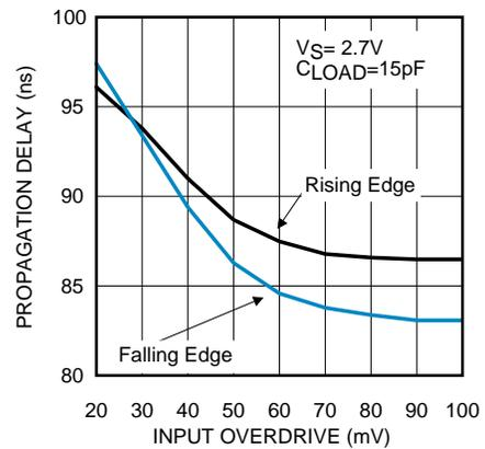
Figure 12. Propagation Delay vs. Input Overdrive
