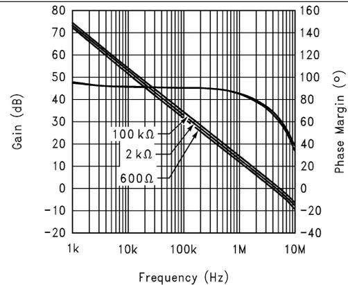
Figure 18. Gain and Phase Margin vs. Frequency ( $R_L = 100k\Omega, 2k\Omega, 600\Omega$ ) at 2.7V
