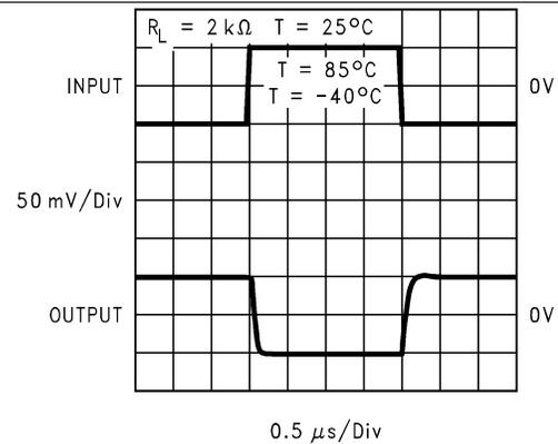
Figure 30. Inverting Small Signal Pulse Response
