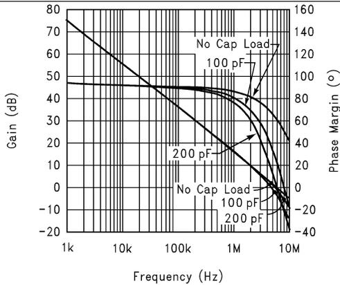
Figure 23. Gain and Phase Margin vs. Frequency ( $C_L = 100pF, 200pF, 0pF$ ,  $R_L = 10k\Omega$ ) at 5V
