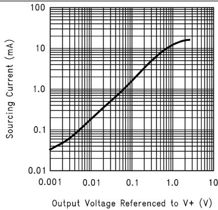
Figure 3. Sourcing Current vs. Output Voltage ( $V_S = 2.7V$ )
