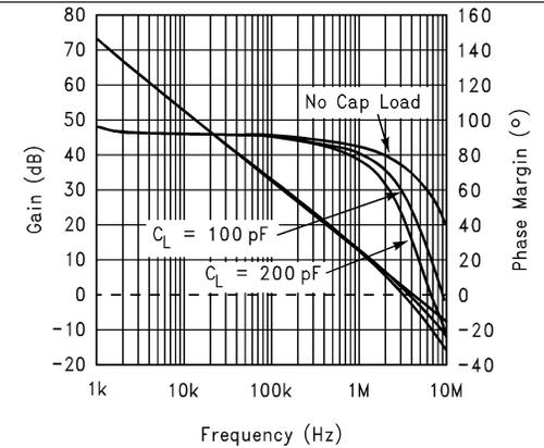
Figure 24. Gain and Phase Margin vs. Frequency ( $C_L = 100pF, 200pF, 0pF$ ,  $R_L = 600\Omega$ ) at 2.7V
