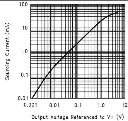
Figure 4. Sourcing Current vs. Output Voltage ( $V_S = 5V$ )
