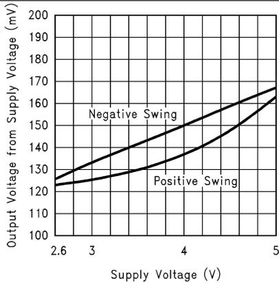
Figure 9. Output Voltage Swing vs. Supply Voltage ( $R_L = 600\Omega$ )
