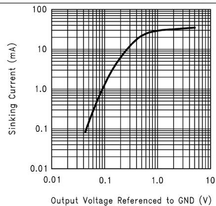
Figure 6. Sinking Current vs. Output Voltage ( $V_S = 5V$ )
