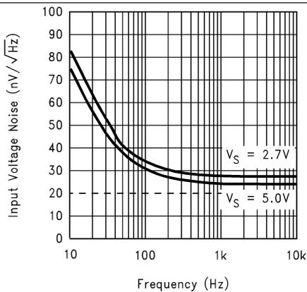
Figure 11. Input Voltage Noise vs. Frequency
