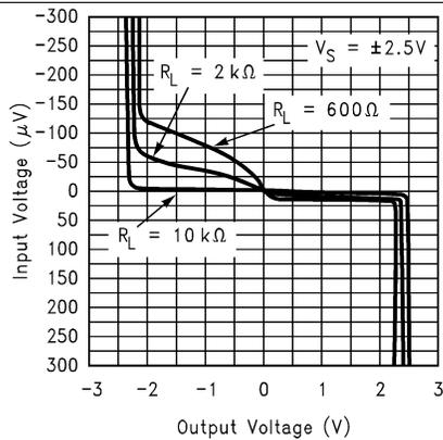
Figure 17. Input Voltage vs. Output Voltage
