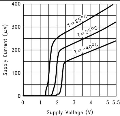
Figure 1. Supply Current vs. Supply Voltage (LMV821)
