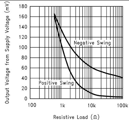
Figure 10. Output Voltage Swing vs. Load Resistance
