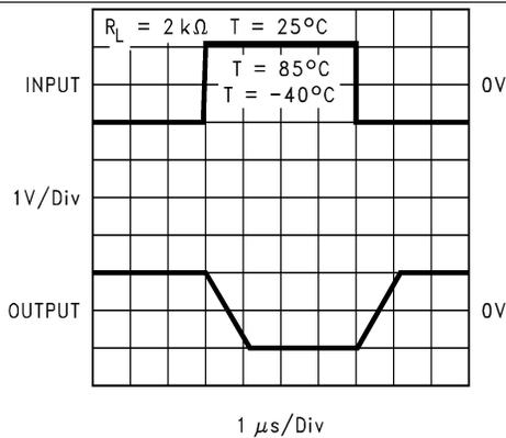
Figure 29. Inverting Large Signal Pulse Response
