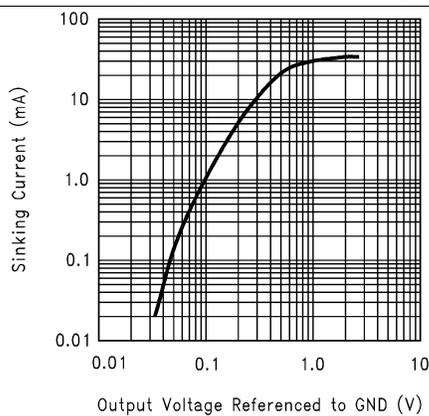
Figure 5. Sinking Current vs. Output Voltage ( $V_S = 2.7V$ )
