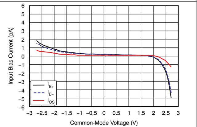
Figure 4. Input Bias Current vs Common-Mode Voltage
