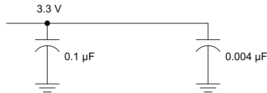
图 9-2. Recommended M-LVDS Bypass Capacitor Layout
