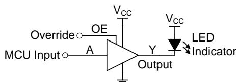
図 16. Application Schematic with MCU driving an LED Indicator
