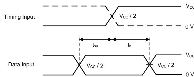
**図 12. Voltage Waveforms: Setup and Hold Times**
