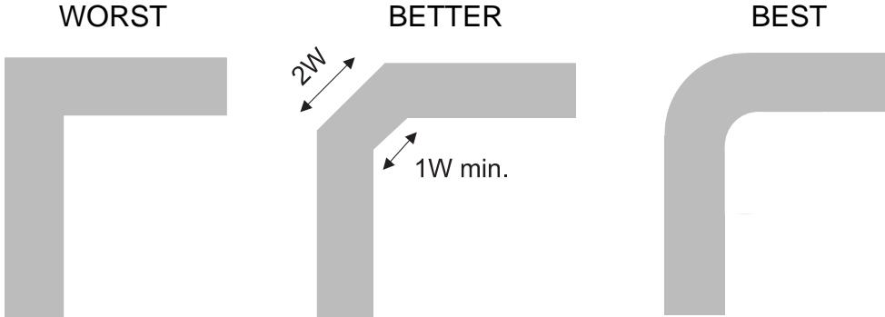
shows progressively better techniques of rounding corners. Only the last example (BEST) maintains constant trace width and minimizes reflections.
