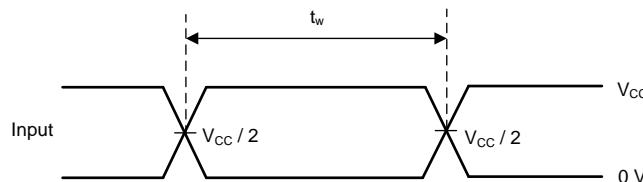
図 10. Voltage Waveforms: Pulse Duration
