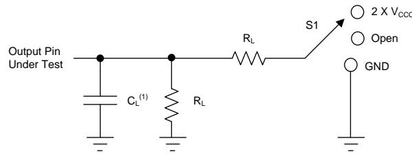
(1)  $C_L$  includes probe and jig capacitance.
