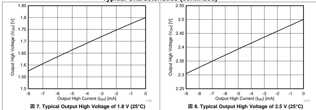
図 7. Typical Output High Voltage of 1.8 V (25°C)
