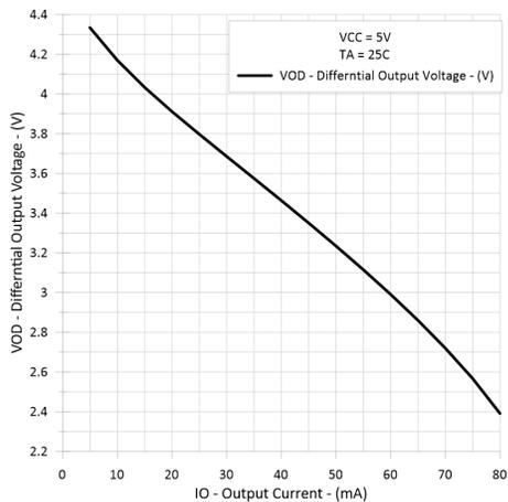
5-3. Driver Differential Output Voltage vs Output Current
