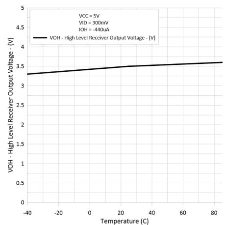
5-5. Receiver High-Level Output Voltage vs Free-Air Temperature
