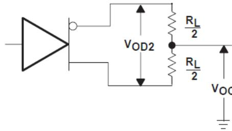
FIG 6-1. Driver  $V_{OD2}$  and  $V_{OC}$
