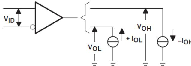
**图 6-6. Receiver VOH and VOL Test Circuit**
