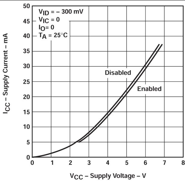
図 5-12. Supply Current vs Supply Voltage
