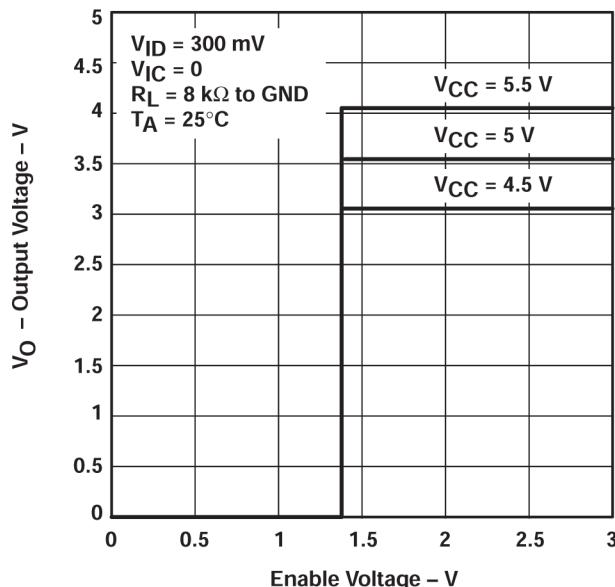
図 5-1. Output Voltage vs Enable Voltage
