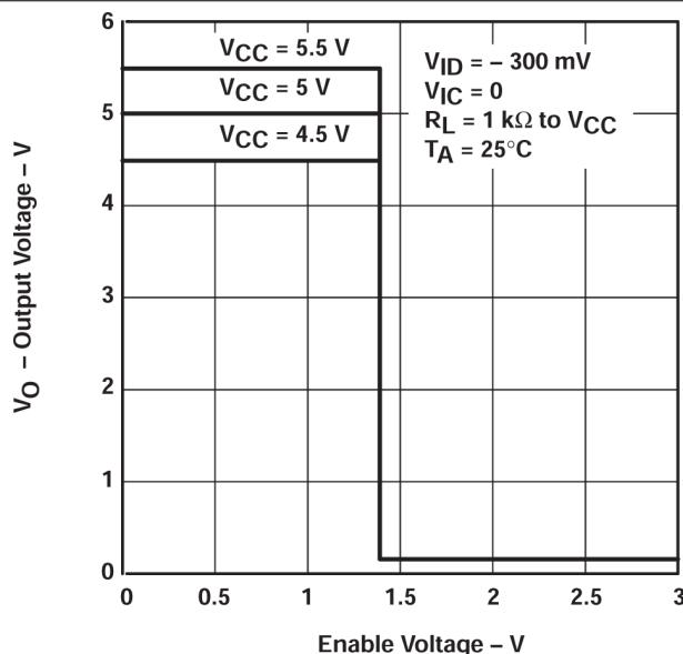
図 5-3. Output Voltage vs Enable Voltage
