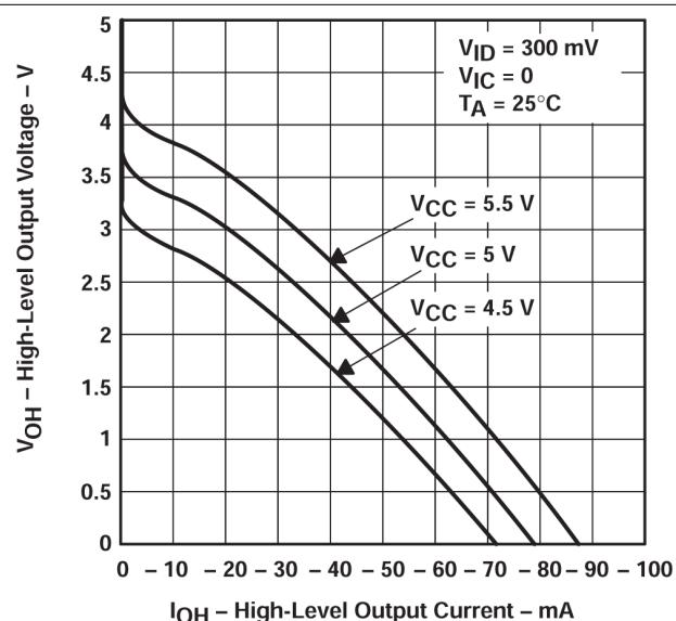
图 5-7. High-level Output Voltage vs High-level Output Current
