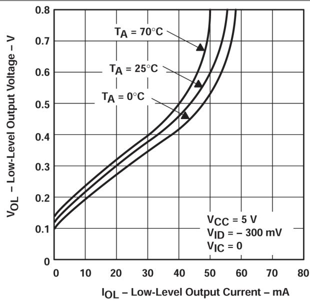
図 5-11. Low-level Output Voltage vs Low-level Output Current
