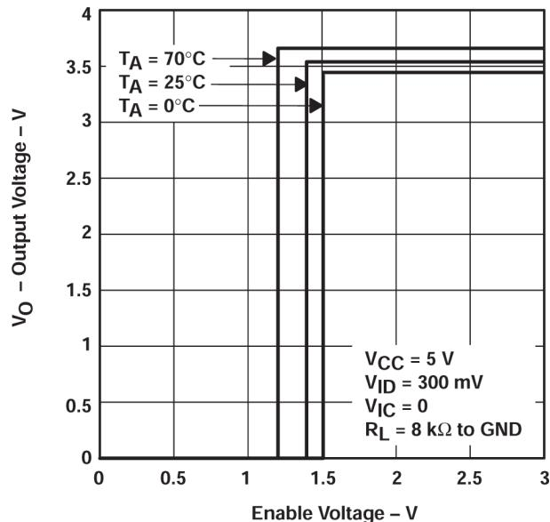
図 5-2. Output Voltage vs Enable Voltage
