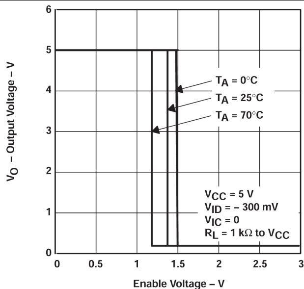
図 5-4. Output Voltage vs Enable Voltage
