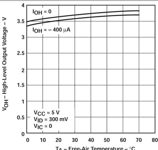
图 5-6. High-level Output Voltage vs Free-air Temperature
