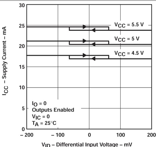
図 5-14. Supply Current vs Differential Input Voltage
