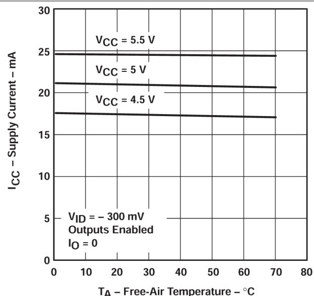
図 5-13. Supply Current vs Free-air Temperature
