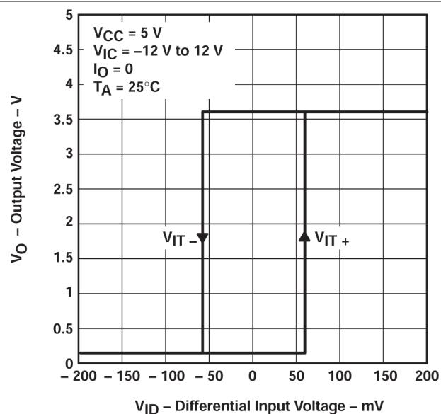
图 5-5. Output Voltage vs Differential Input Voltage
