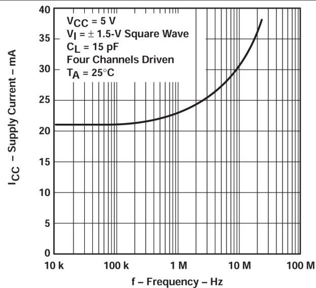
図 5-15. Supply Current vs Frequency
