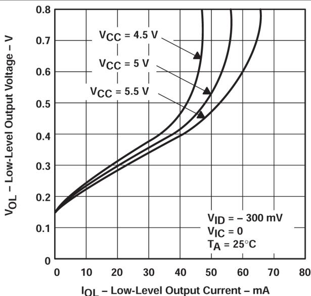
図 5-10. Low-level Output Voltage vs Low-level Output Current
