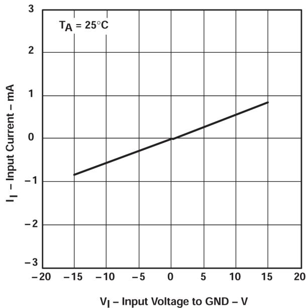
図 5-17. Input Current vs Input Voltage to Gnd
