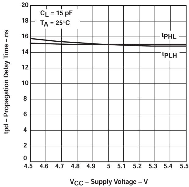
図 5-19. Propagation Delay Time vs Supply Voltage
