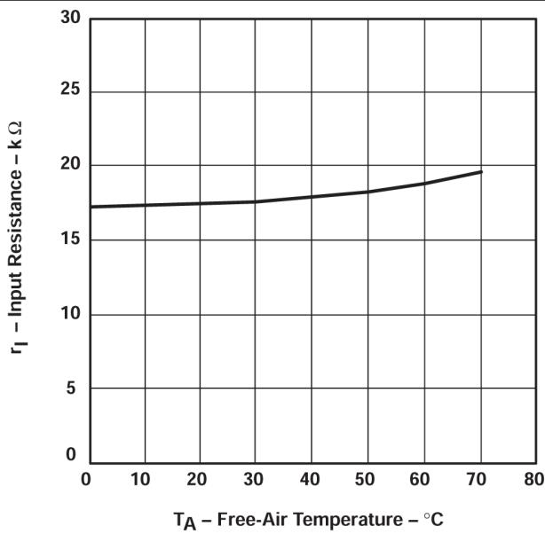
図 5-16. Input Resistance vs Free-air Temperature
