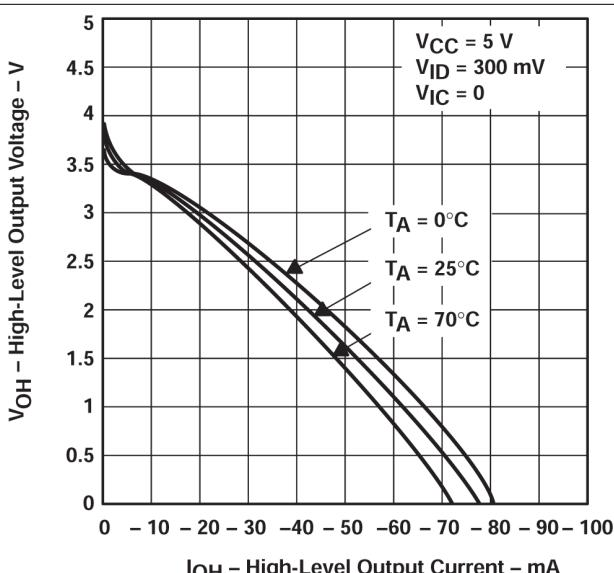
图 5-8. High-level Output Voltage vs High-level Output Current
