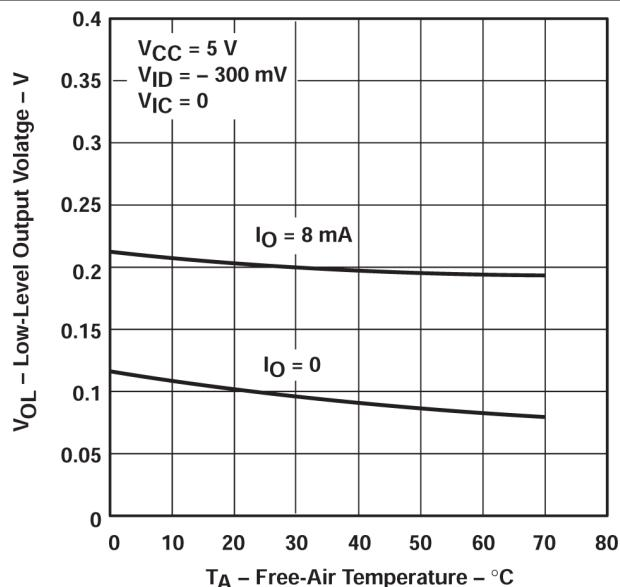
図 5-9. Low-level Output Voltage vs Free-air Temperature
