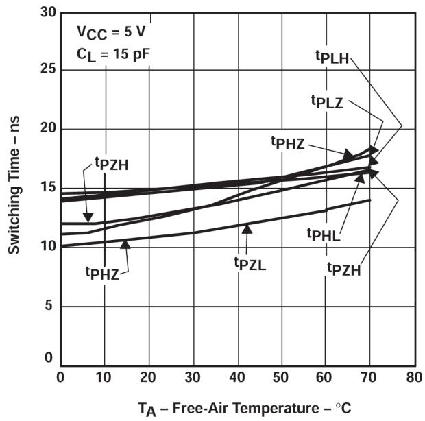
図 5-18. Switching Time vs Free-air Temperature
