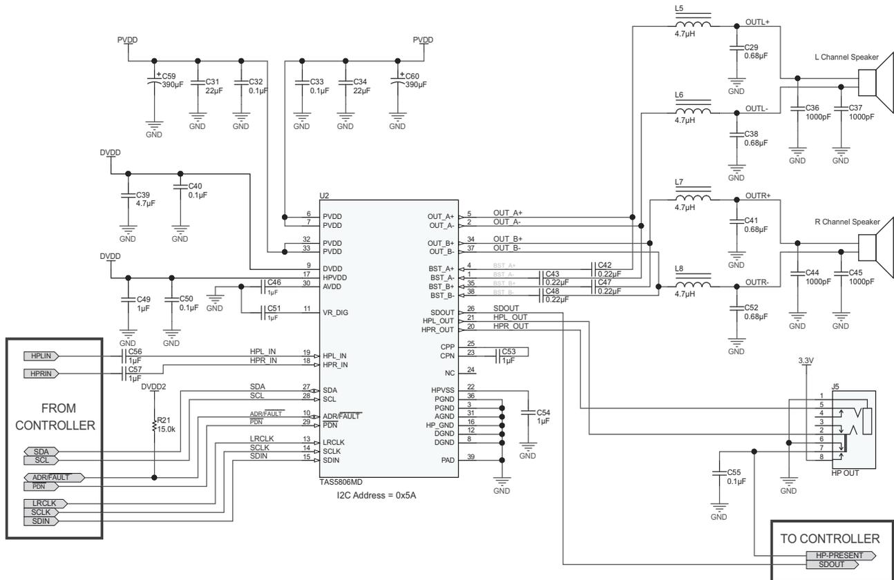
127. 2.0 (Stereo BTL) System Application Schematic
