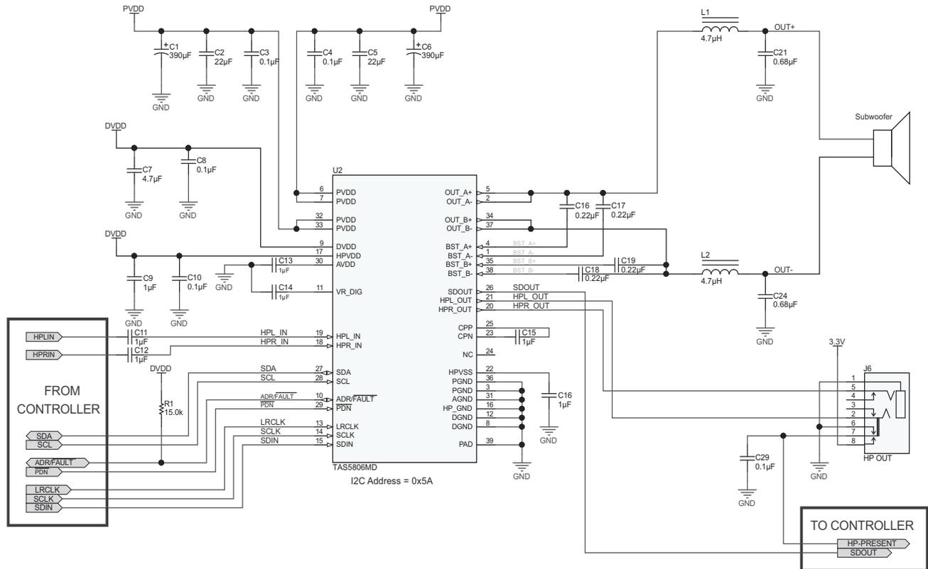
FIG 134. Mono (PBTL) System Application Schematic
