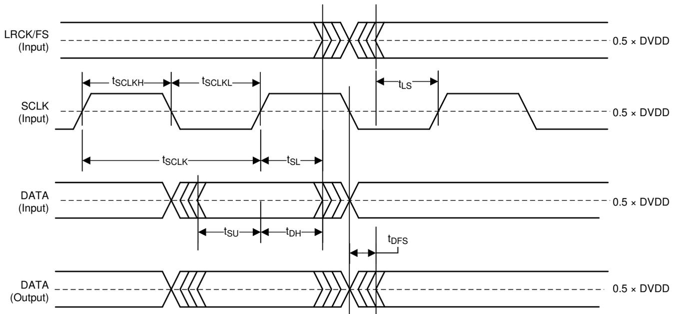
图 64. Serial Audio Port Timing in Slave Mode
