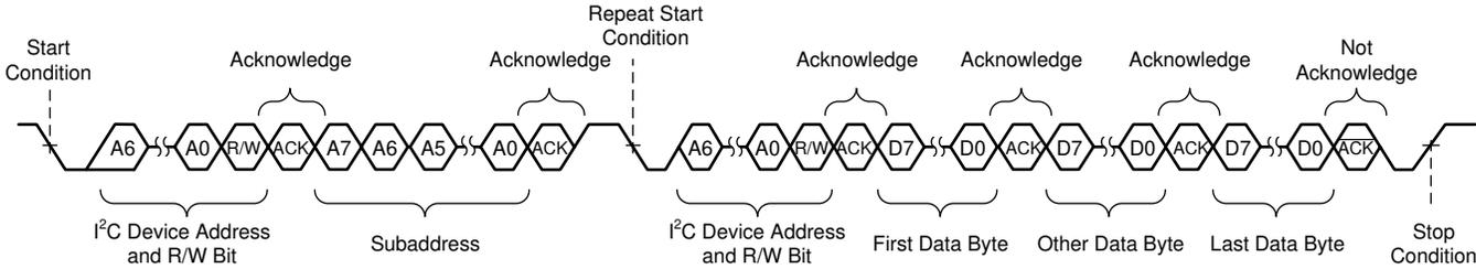
79. Except for the last data byte, the master device responds with an acknowledge bit after receiving each data byte and automatically increments the I<sup>2</sup>C sub address by one. After receiving the last data byte, the master device transmits a not-acknowledge followed by a stop condition to complete the transfer.
