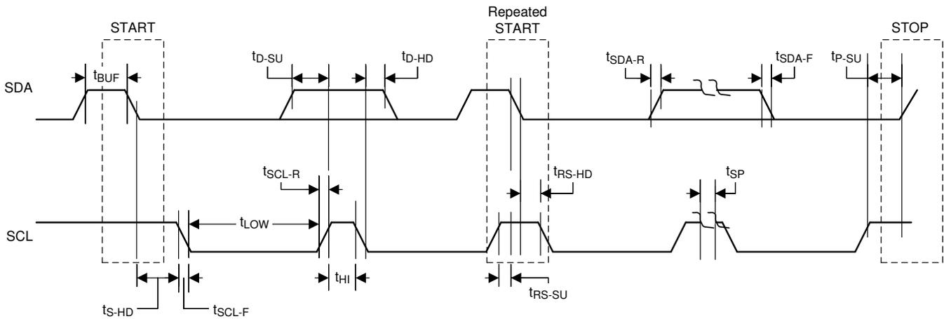
图 65. I<sup>2</sup>C Communication Port Timing Diagram
