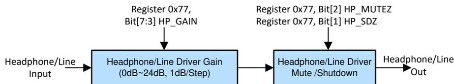
**图 73. Headphone/Line driver control with I<sup>2</sup>C**
