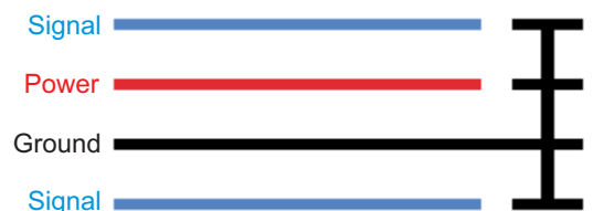
Figure 8-13. Guard Ring Routing
