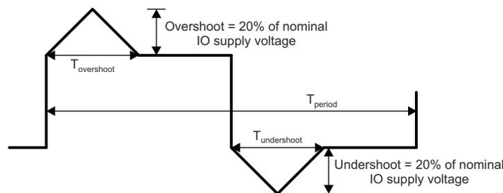
A.  $T_{\text{overshoot}} + T_{\text{undershoot}} < T_{\text{period}}$  の 20%
