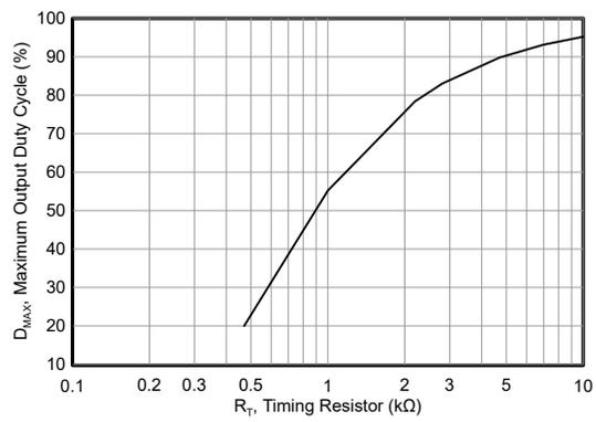
**図 5-9. Maximum Output Duty Cycle vs Timing Resistor**
