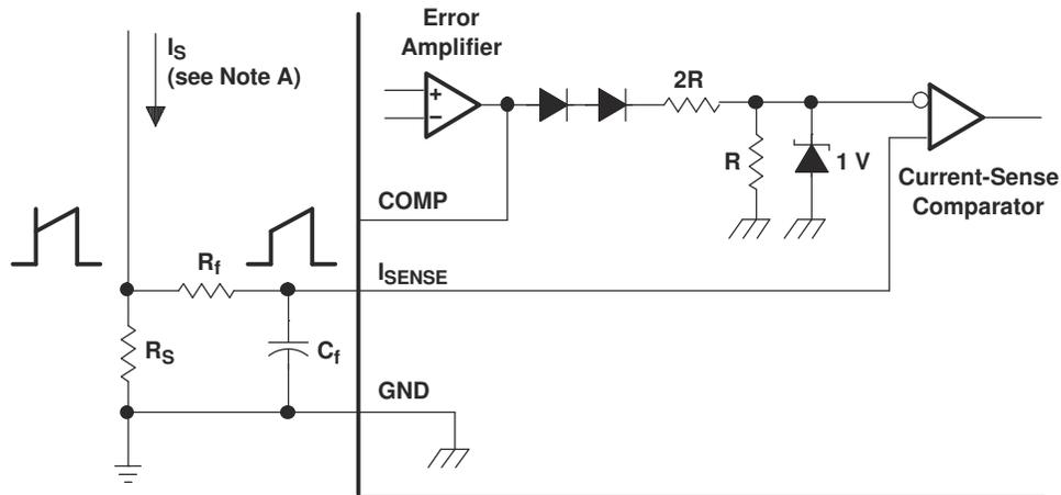
A. Peak current ( $I_S$ ) is determined by the formula:  $I_{S(max)} = 1 V/R_S$
