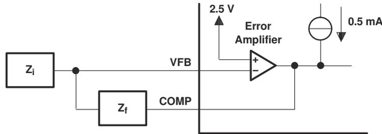
A. Error amplifier can source or sink up to 0.5 mA.
