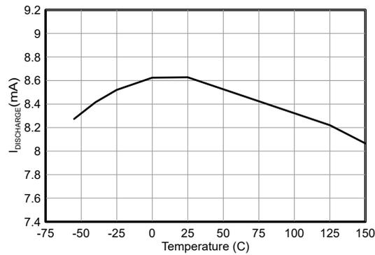
図 5-4. Oscillator Discharge Current vs Temperature
