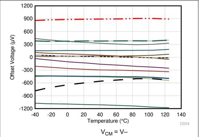
6-4. Offset Voltage vs Temperature
