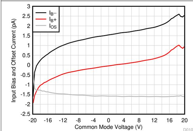
Figure 6-9. Input Bias Current vs Common-Mode Voltage
