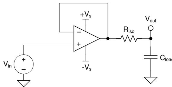
**Figure 7-8. Extending Capacitive Load Drive With the TLV9301**
