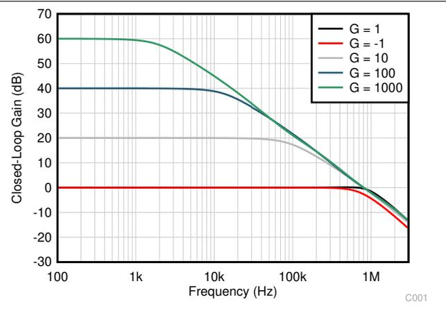
Figure 6-8. Closed-Loop Gain and Phase vs Frequency
