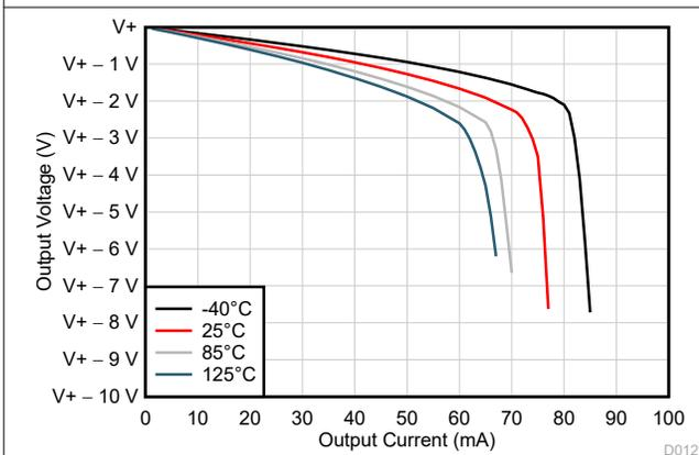
Figure 6-11. Output Voltage Swing vs Output Current (Sourcing)
