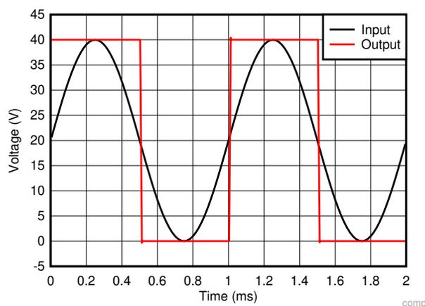
图 8-2. Comparator Output Response to Input Voltage
