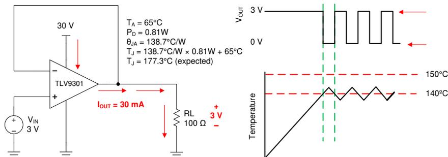
**Figure 7-5. Thermal Protection**
