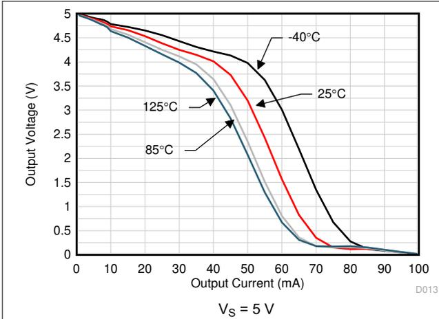
**6-13. Output Voltage Swing vs Output Current (Sourcing)**
