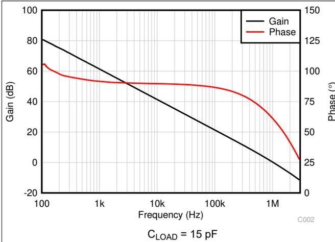
Figure 6-7. Open-Loop Gain and Phase vs Frequency
