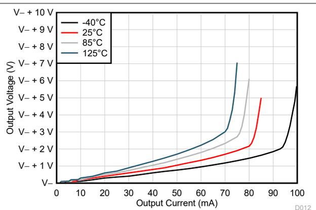
Figure 6-12. Output Voltage Swing vs Output Current (Sinking)
