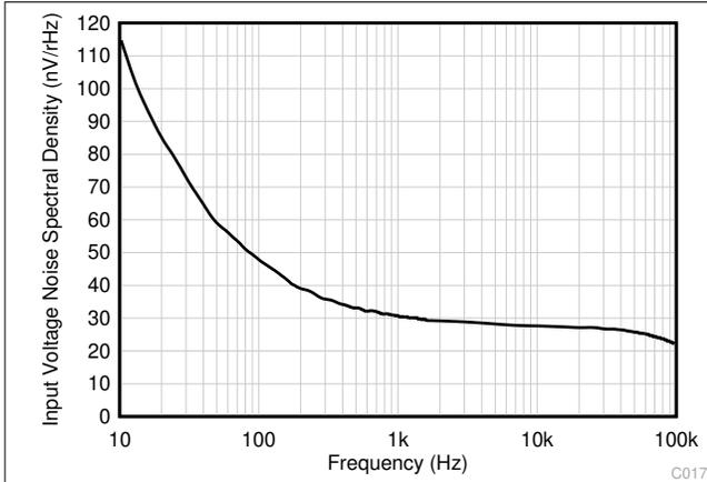
6-19. Input Voltage Noise Spectral Density vs Frequency
