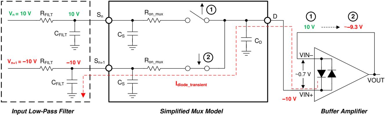
7-2. For low-gain circuits, these fast-ramping input signals forward-bias back-to-back diodes, causing an increase in input current and resulting in extended settling time.
