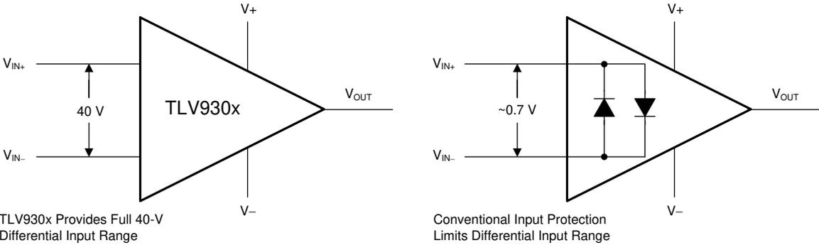
7-1. TLV930x Input Protection Does Not Limit Differential Input Capability
