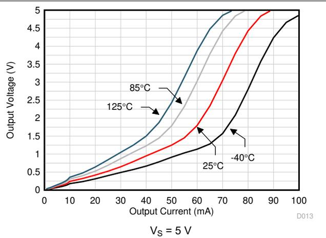
**6-14. Output Voltage Swing vs Output Current (Sinking)**
