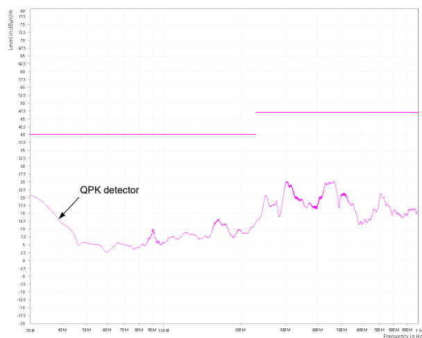
Figure 9-10. CISPR 32 Class B Radiated Emissions: Horizontal Polarization
