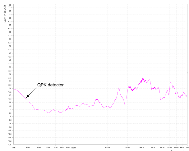
Figure 9-11. CISPR 32 Class B Radiated Emissions: Vertical Polarization
