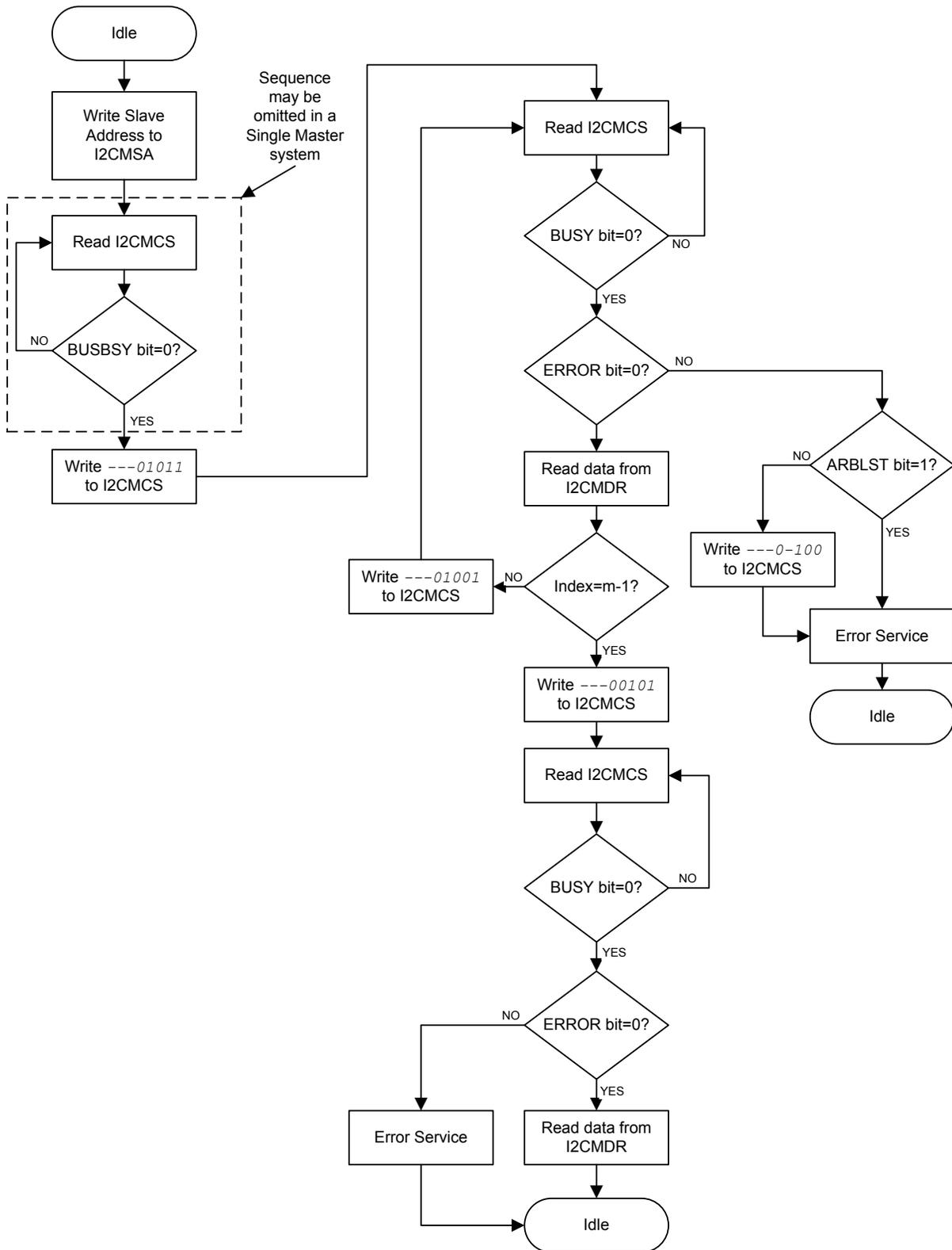
Figure 18-12. Master RECEIVE with Repeated START after Master TRANSMIT
