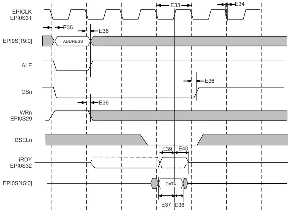
Figure 27-27. PSRAM Single Burst Write
