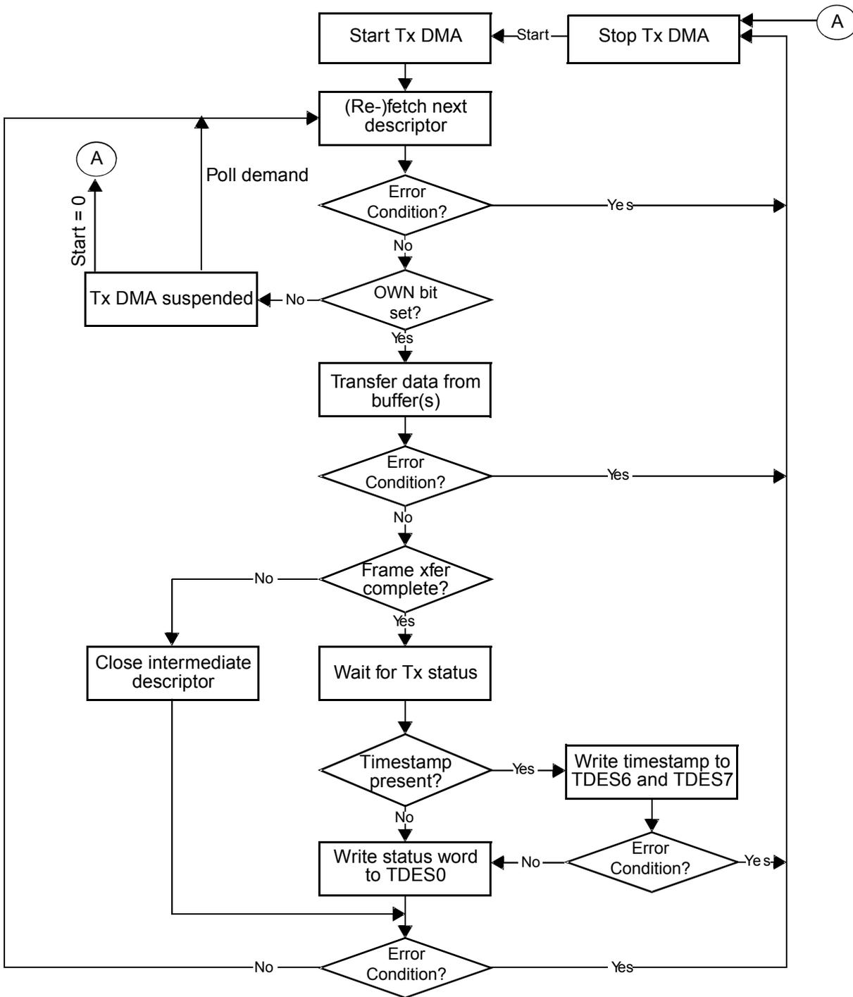
**TX DMA OSF Mode Operation**
