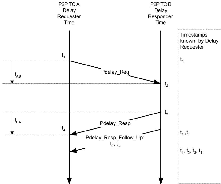
As shown in Figure 20-11 on page 1450, the propagation delay is calculated in the following way:
