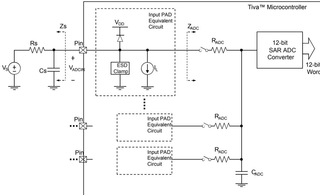
The ADC operates from both the 3.3-V analog and 1.2-V digital power supplies. The ADC clock can be configured to reduce power consumption when ADC conversions are not required (see “System Control” on page 239). The analog inputs are connected to the ADC through specially balanced input paths to minimize the distortion and cross-talk on the inputs. Detailed information on the ADC power supplies and analog inputs can be found in “Analog-to-Digital Converter (ADC)” on page 1815.
