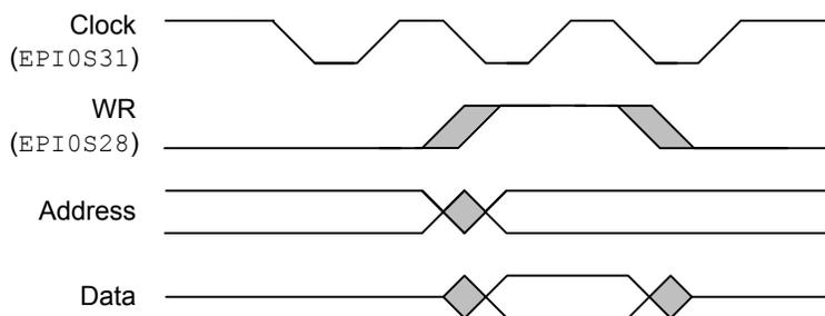
**Figure 11-29. EPI Clock Operation, CLKGATE=1, WR2CYC=1**
