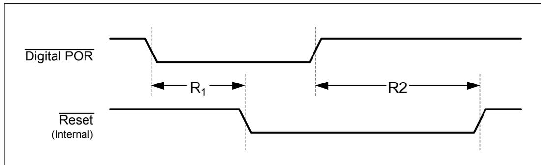
The digital Power-On Reset is only released when the analog Power-On Reset has deasserted and all of the Power-OK monitors for each of the supplies indicate that power levels are in operational ranges.
