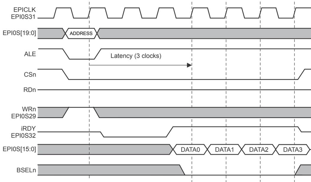
Figure 11-8. PSRAM Burst Write
