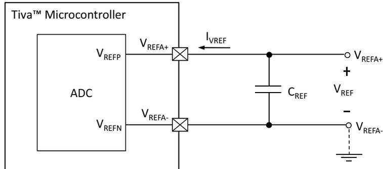
Figure 27-29. ADC Input Equivalency
