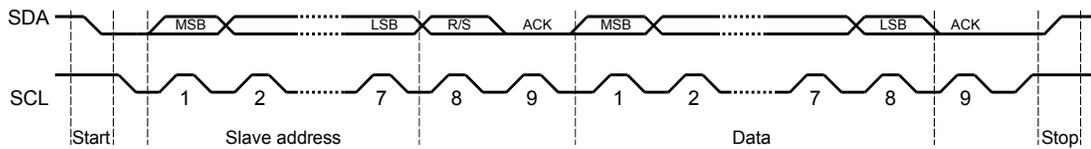
The first seven bits of the first byte make up the slave address (see Figure 18-5). The eighth bit determines the direction of the message. A zero in the R/S position of the first byte means that the master transmits (sends) data to the selected slave, and a one in this position means that the master receives data from the slave.
