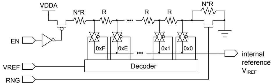
**Note:** In the figure above,  $N \cdot R$  represents a multiple of the  $R$  value that produces the results specified in Table 22-2 on page 1594.
