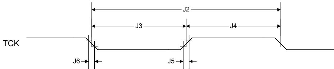
Figure 27-3. JTAG Test Access Port (TAP) Timing
