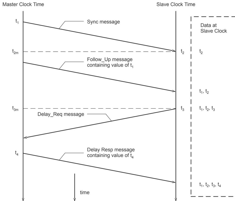
As shown in Figure 20-9 on page 1445, the PTP uses the following process:
