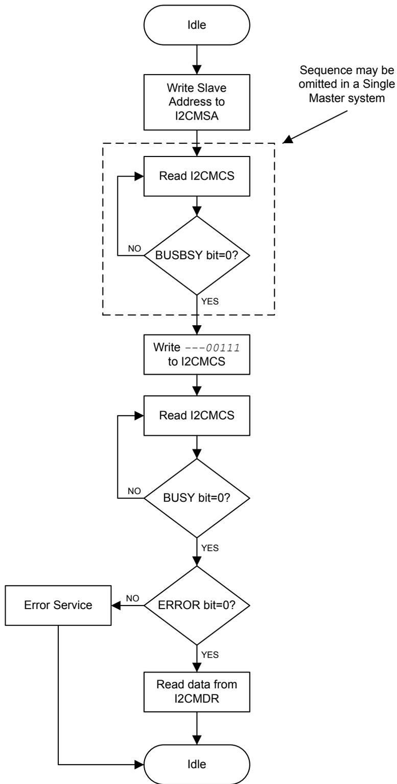
Figure 18-10. Master TRANSMIT of Multiple Data Bytes
