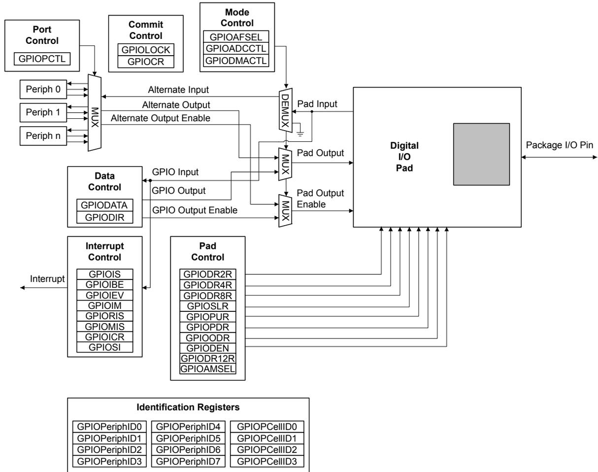
Figure 10-2. Analog/Digital I/O Pads
