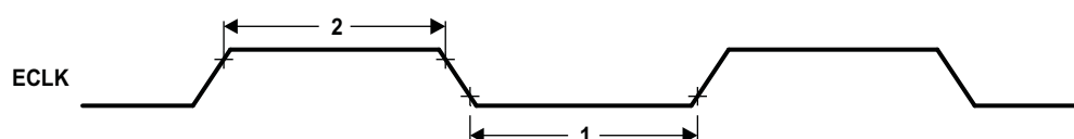
Figure 5-7. ECLK Timing Diagram
