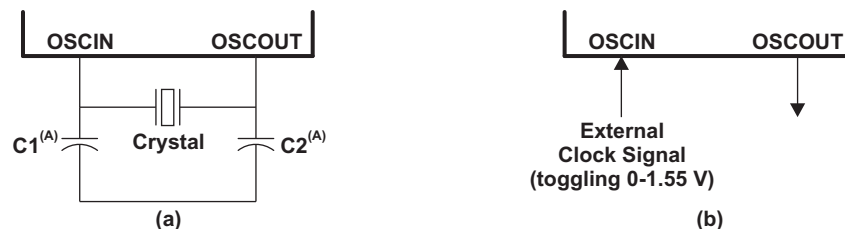
Figure 5-3. Recommended Crystal/Clock Connection
