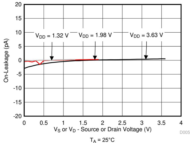
Figure 9-5. On-Leakage vs Source or Drain Voltage
