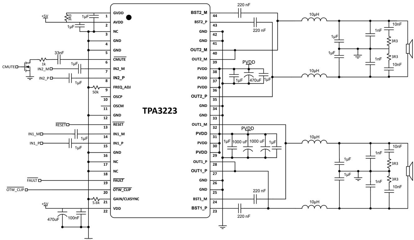
図 10-1. Typical Differential (2N) AD-Mode BTL Application
