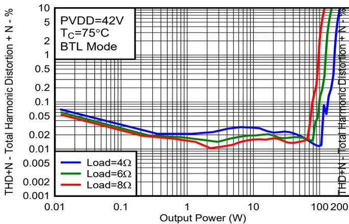
**10-2. Total Harmonic Distortion + Noise vs Output Power**
