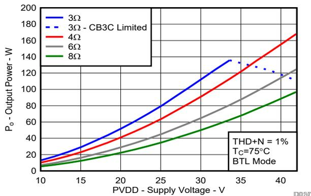
7-5. Output Power vs Supply Voltage, AD-mode
