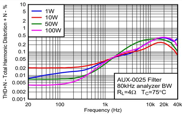
7-3. Total Harmonic Distortion+Noise vs Frequency
