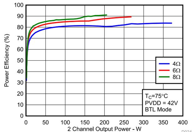
7-6. System Efficiency vs Output Power
