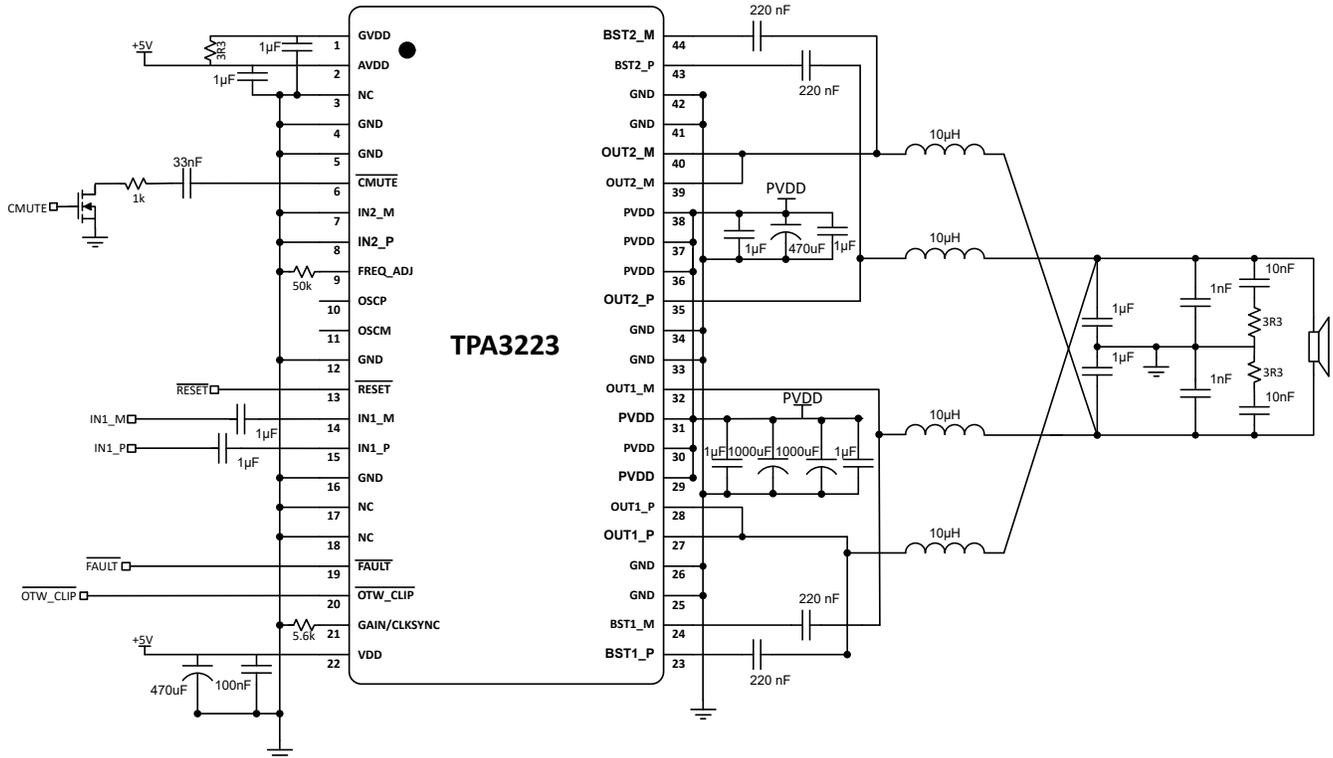
图 10-6. Typical Differential (2N) AD-Mode PBTL Application
