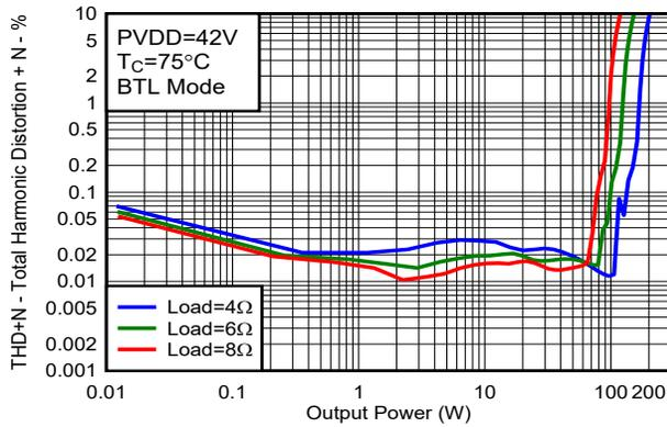
7-1. Total Harmonic Distortion + Noise vs Output Power
