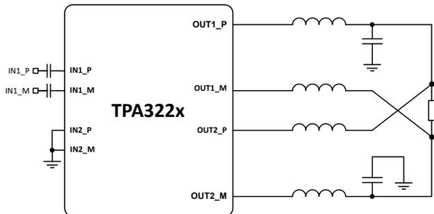
**图 9-12. Mono PBTL, Post LC Filter**
