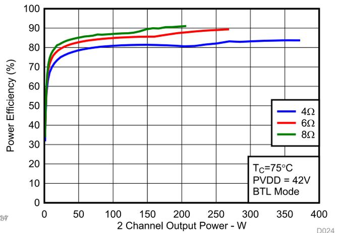
**10-5. System Efficiency vs Output Power**
