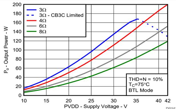
7-4. Output Power vs Supply Voltage, AD-mode
