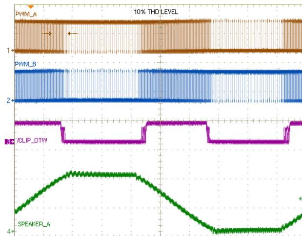
9-15. Signal Clipping PWM and Speaker Output Signals
