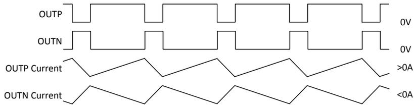
9-8. AD Mode Output Waveforms, High Level Output
