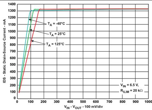
17. Switch Current Vs. Drain-Source Voltage Across Switch
