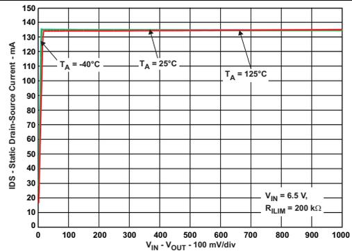
18. Switch Current Vs. Drain-Source Voltage Across Switch
