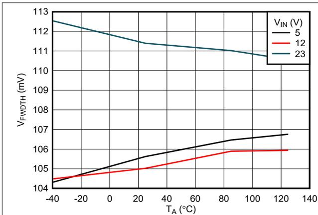
6-19. RCB - Forward Comparator Threshold vs Temperature
