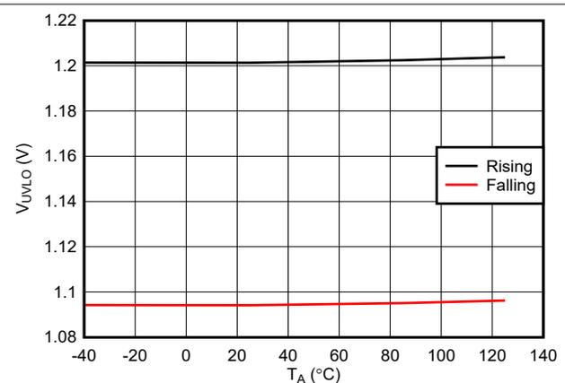
图 6-10. EN/UVLO FET Turn OFF Threshold vs Temperature
