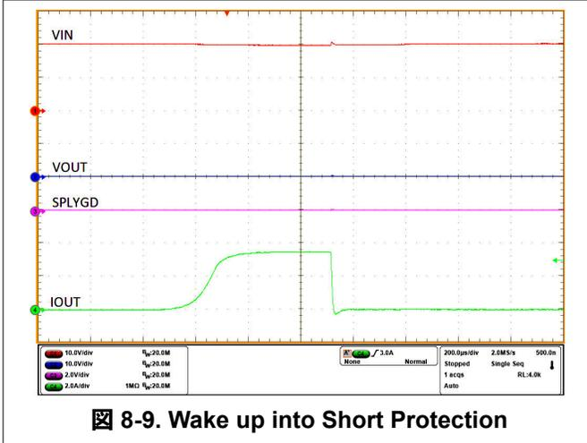
図 8-9. Wake up into Short Protection
