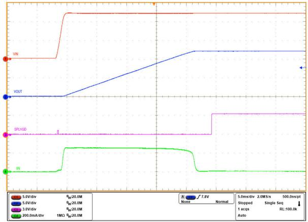
V<sub>EN/UVLO</sub> = 2 V, C<sub>OUT</sub> = 220 μF, C<sub>dVdt</sub> = 10 nF, V<sub>IN</sub> ramped up to 12 V
