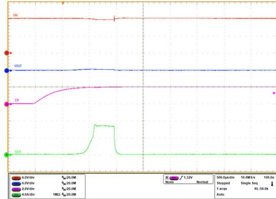
$V_{IN} = 12\text{ V}$ , OUT short-circuit to GND,  $I_{LIM}$  set to 4.5 A,  $V_{EN/UVLO}$  stepped from 0 V to 2 V
