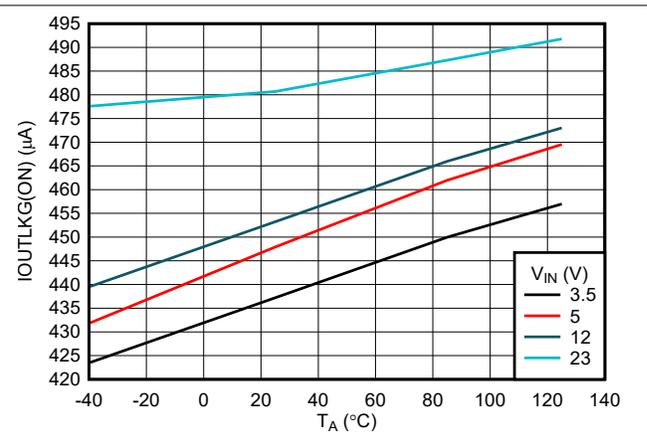
6-20. OUT Leakage Current During ON-State Reverse Current Blocking
