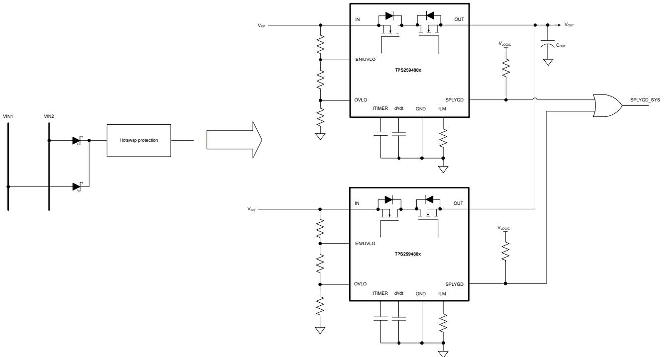
図 8-11. Two Devices, Active ORing Configuration
