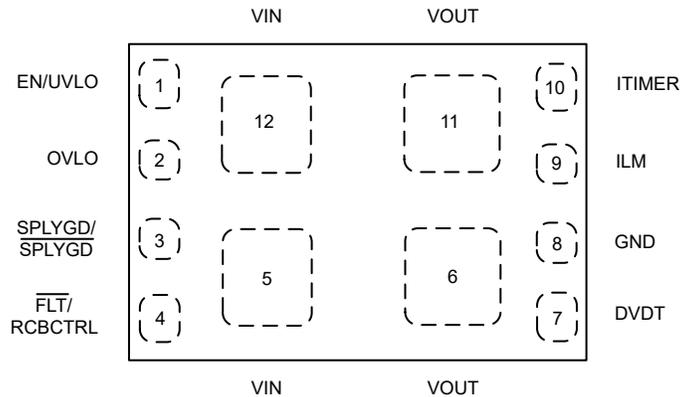
図 5-1. YWP Package, 12-Ball PWCSOP (Top View)
