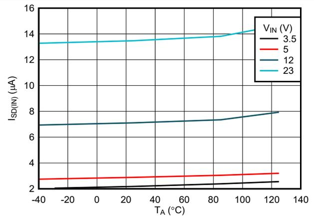
6-4. IN Shutdown Current vs Temperature
