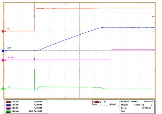
C<sub>IN</sub> = 0.1 μF, C<sub>OUT</sub> = 220 μF, C<sub>dVdt</sub> = 10 nF, EN/UVLO connected to IN through resistor ladder, 12 V hot-plugged to IN
