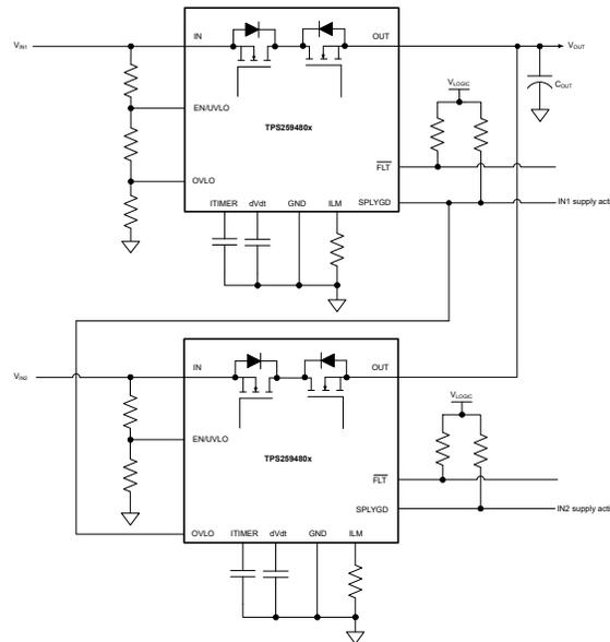
图 8-14. Priority Power MUXing With 2 x TPS259480x - Option 1
