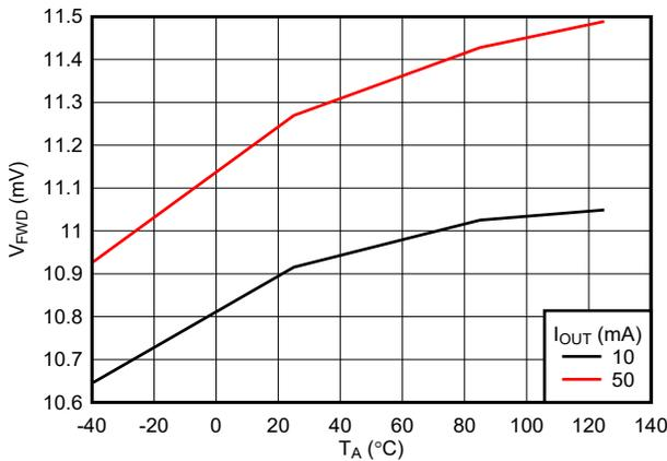
Figure 6-17. RCB - Forward Regulation Voltage vs Temperature
