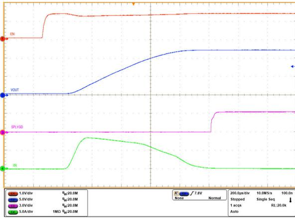
V<sub>IN</sub> = 12 V, C<sub>OUT</sub> = 220 μF, C<sub>dVdt</sub> = Open, V<sub>EN/UVLO</sub> stepped up to 2 V
