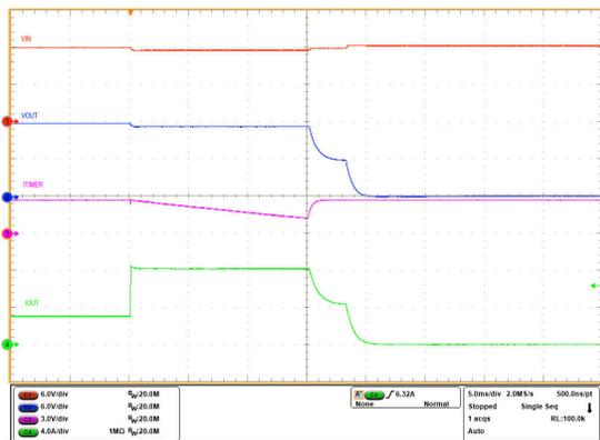
$V_{IN} = 12\text{ V}$ ,  $C_{TIMER} = 22\ \text{nF}$ ,  $C_{OUT} = 220\ \mu\text{F}$ ,  $I_{LIM}$  set to 4.5 A,  $I_{OUT}$  stepped from 3 A → 9 A
