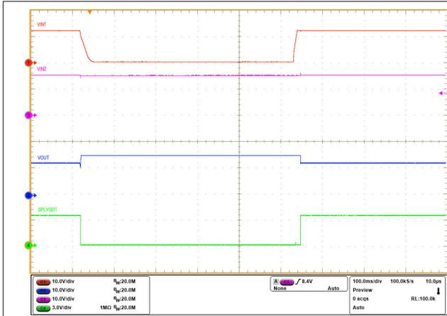
図 8-15. TPS259480x Power MUX - Switchover Between Primary and Auxiliary Supplies
