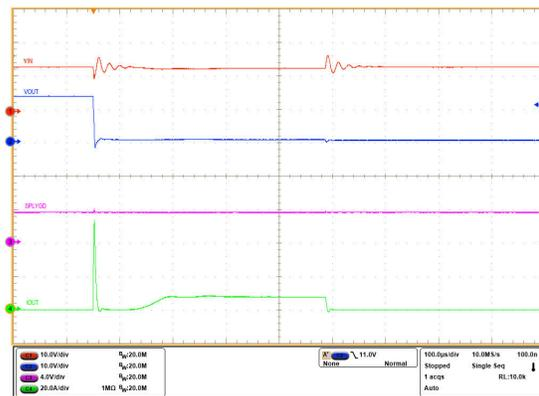
$V_{IN} = 12\text{ V}$ ,  $I_{LIM}$  set to 9 A,  $V_{EN/UVLO} = 2\text{ V}$ ,  $I_{OUT}$  stepped from Open → Short-circuit to GND
