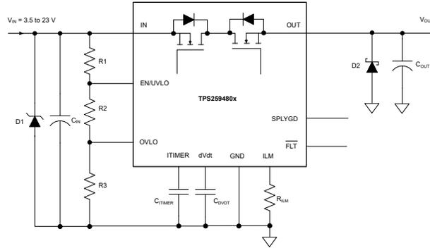
図 8-23. Circuit Implementation with Optional Protection Components
