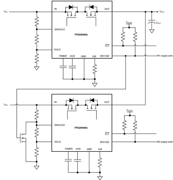
図 8-18. Priority Power MUXing With 2 × TPS25948x - Option 3
