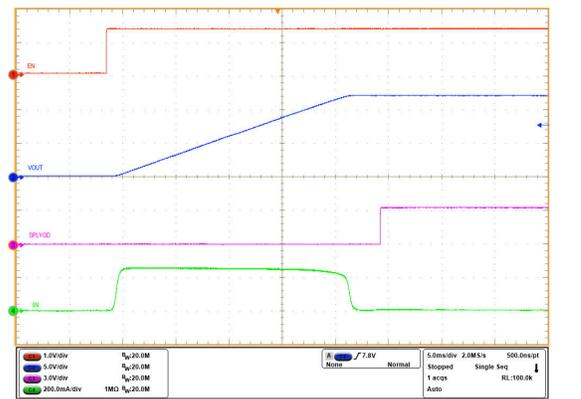
V<sub>IN</sub> = 12 V, C<sub>OUT</sub> = 220 μF, C<sub>dVdt</sub> = 10 nF, V<sub>EN/UVLO</sub> stepped up to 2 V
