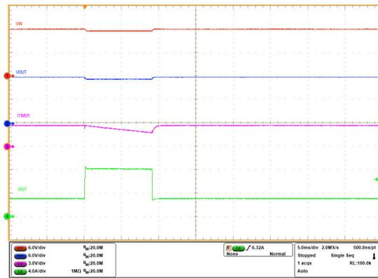
$V_{IN} = 12\text{ V}$ ,  $C_{TIMER} = 22\ \text{nF}$ ,  $C_{OUT} = 220\ \mu\text{F}$ ,  $I_{LIM}$  set to 4.5 A,  $I_{OUT}$  ramped from 3 A → 8 A → 3 A within 9 ms
