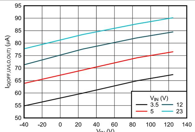
6-6. OUT OFF State (UVLO) Current vs Temperature
