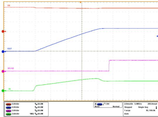
$V_{IN} = 12\text{ V}$ ,  $C_{OUT} = 690\ \mu\text{F}$ ,  $R_{OUT} = 4\ \Omega$ ,  $C_{dVdt} = 3300\ \text{pF}$ ,  $V_{EN/UVLO}$  stepped up to 2 V
