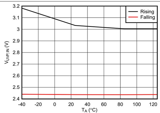
图 6-8. IN Undervoltage Threshold vs Temperature
