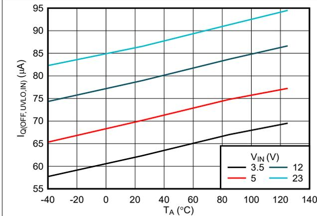
6-3. IN OFF state (UVLO) current vs Temperature
