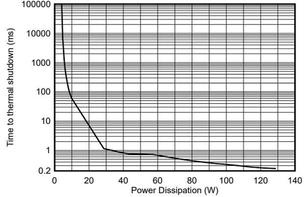
6-26. Time to Thermal Shut-Down During Inrush State
