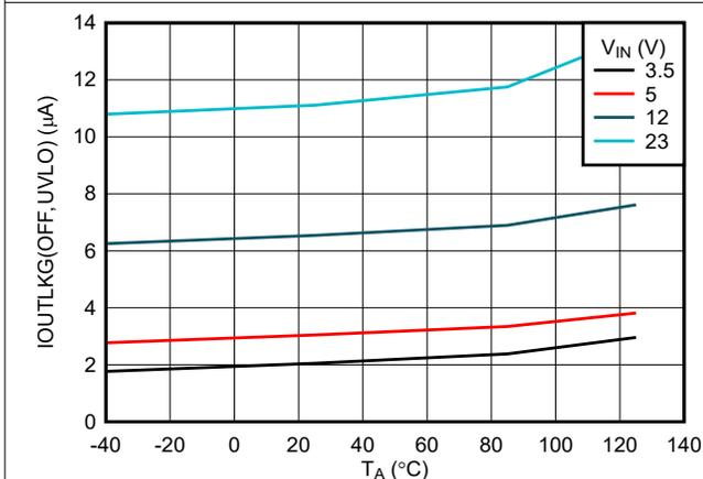
6-21. Reverse Leakage Current During OFF-State
