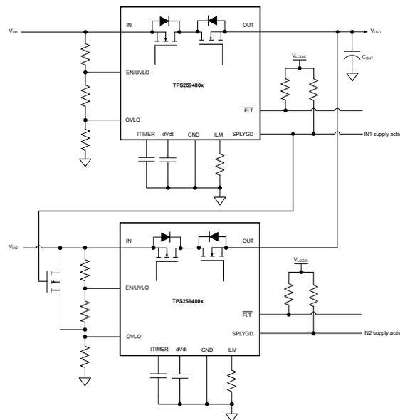
図 8-17. Priority Power MUXing With 2 x TPS259480x - Option 2
