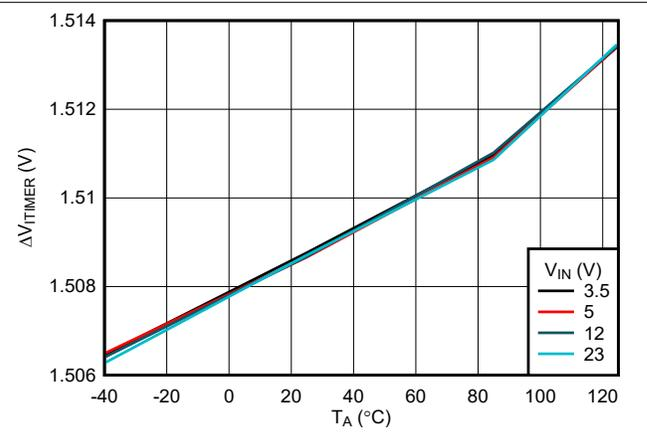
6-22. ITIMER Discharge Differential Voltage Threshold vs Temperature
