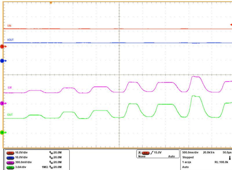
$V_{IN} = 12\text{ V}$ ,  $C_{OUT} = 220\ \mu\text{F}$ ,  $R_{ILM} = 536\ \Omega$ ,  $I_{OUT}$  varied dynamically between 3 A and 8 A
