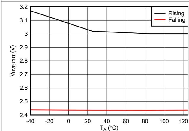
图 6-9. OUT Undervoltage Threshold vs Temperature
