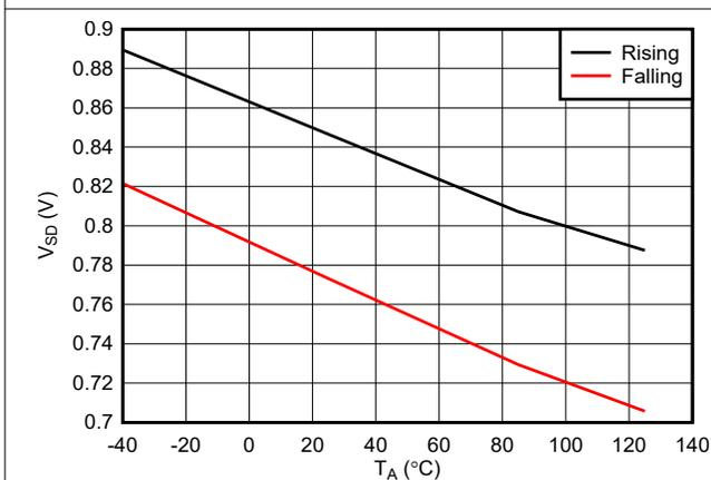
图 6-11. EN/UVLO Shutdown Threshold vs Temperature
