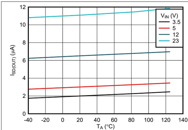
图 6-7. OUT Shutdown Current vs Temperature
