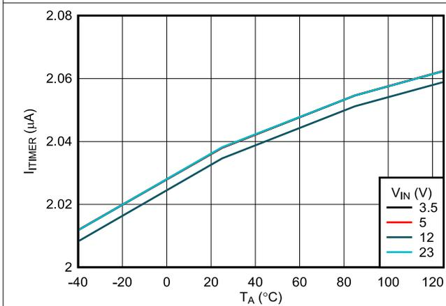
6-23. ITIMER Discharge Current vs Temperature
