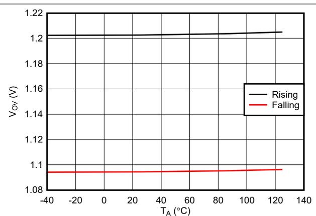
图 6-12. OVLO Threshold vs Temperature
