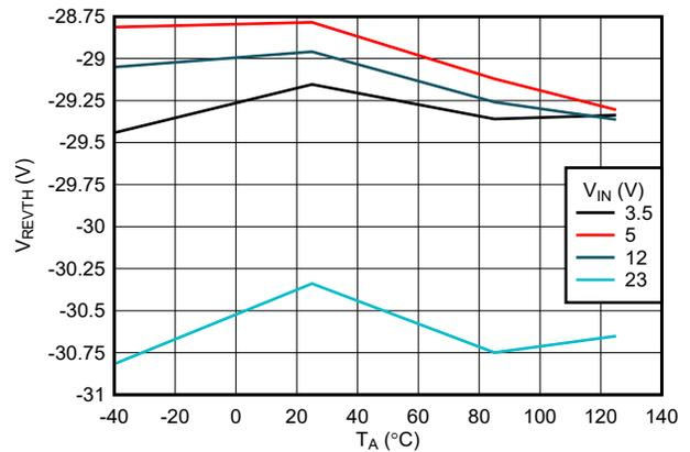
Figure 6-18. RCB - Reverse Comparator Threshold vs Temperature
