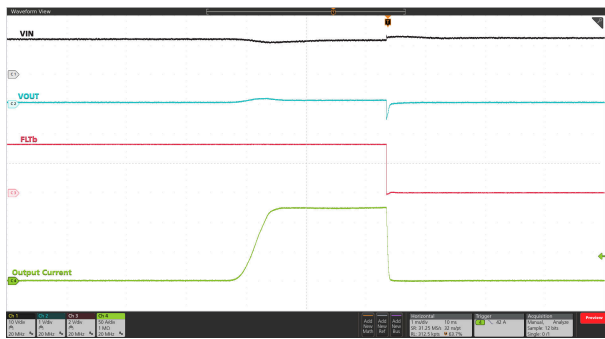
9-7. Power Up into Short: V_{IN} = 12 V, EN/UVLO Stepped Up From 0 V to 3 V, V_{IREF} = 1 V, R_{ILIM(TPS25990)} = 422 \Omega , R_{ILIM(TPS25985)} = 316 \Omega , and OUT Shorted to GND
