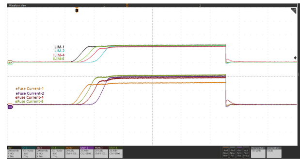
9-8. Power Up into Short (Current distribution among six devices in parallel): V_{IN} = 12 V, EN/UVLO Stepped Up From 0 V to 3 V, V_{IREF} = 1 V, R_{ILIM(TPS25990)} = 422 \Omega , R_{ILIM(TPS25985)} = 316 \Omega , and OUT Shorted to GND
