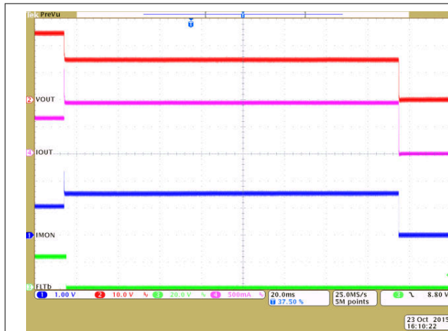
RILIM = 12 k \Omega RILIM = 12 k \Omega Load transient event MODE pin connected from 37 \Omega to 15 \Omega to RTN
