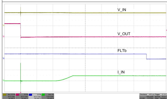
Figure 27. OVP Overvoltage Cut-Off Response
