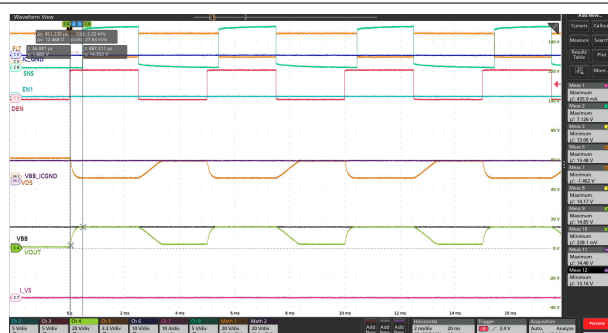
VBB = 13.5V VOUT = 開放負荷 TAMB = 25°C DIAG_EN = PWM VEN1 = 0V SEL = 0 (200Hz)
