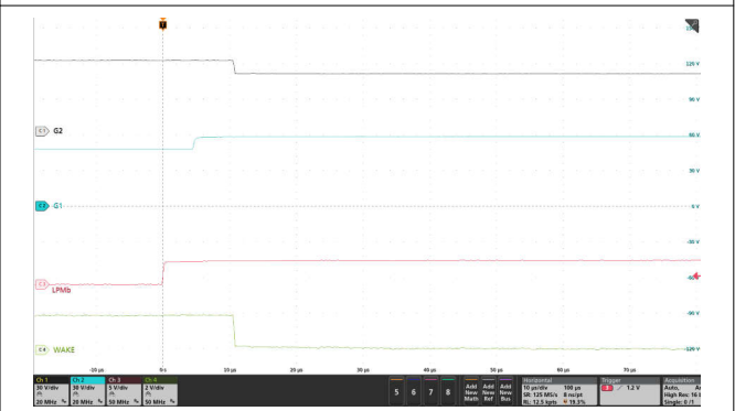
図 8-5. State Transition From LPM to Active Mode (LPM = Low to High, VIN = 48V, No Load)
