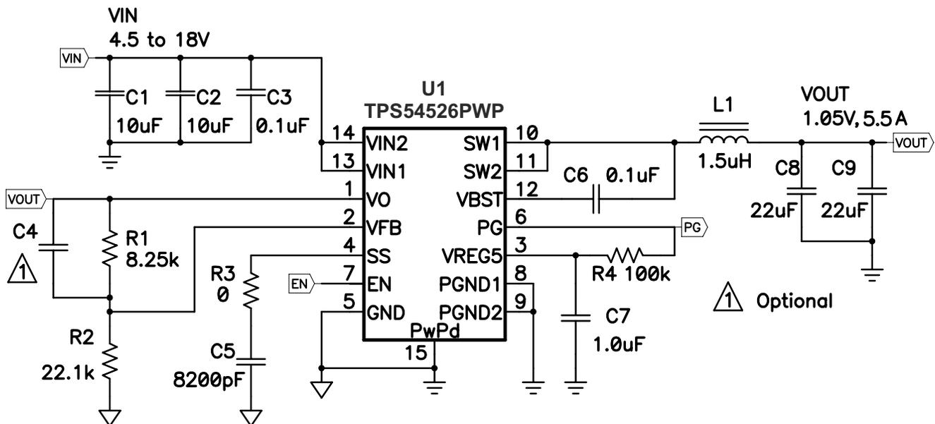
图 8-1. Schematic Diagram for This Design Example
