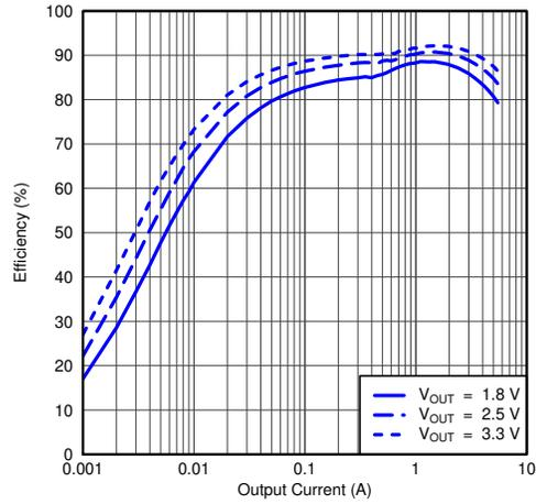
**8-5. Light Load Efficiency vs Output Current**
