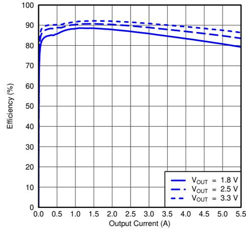
**8-4. Efficiency vs Output Current**
