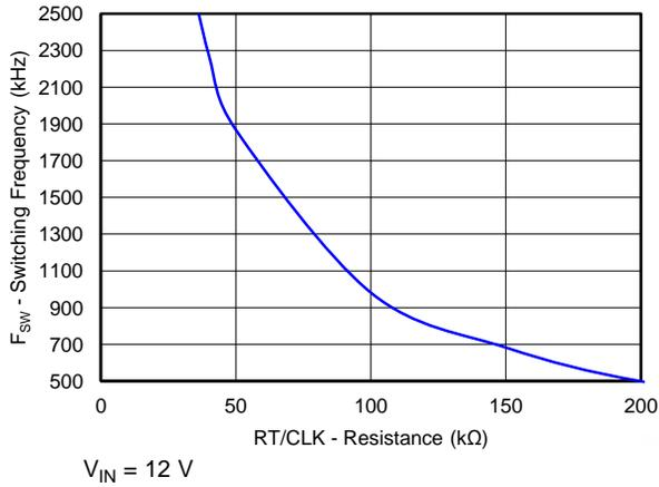
Figure 7. Switching Frequency vs RT/CLK Resistance
