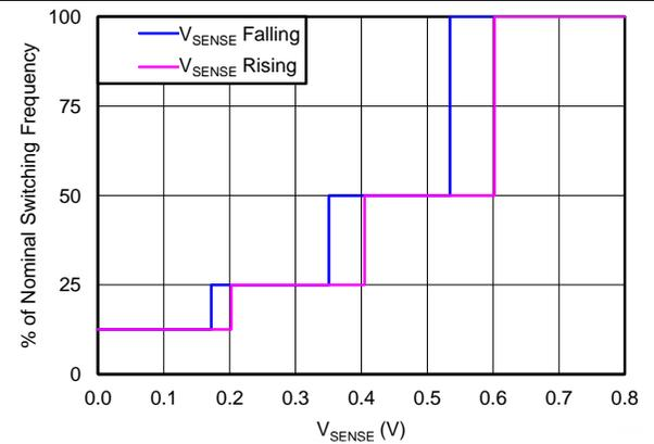
Figure 14. Switching Frequency vs V<sub>SENSE</sub>
