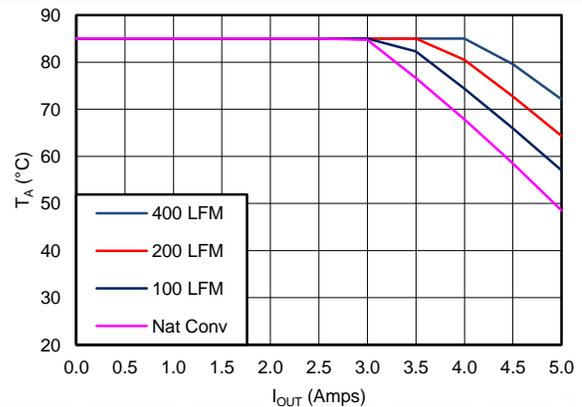
**Figure 55. Air Flow Conditions
