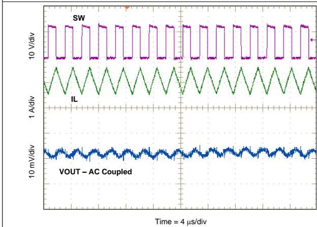
Figure 38. Output Ripple CCM
