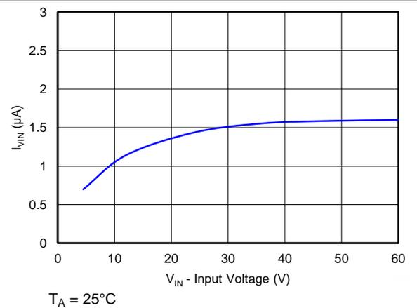
Figure 16. Shutdown Supply Current vs Input Voltage (V<sub>IN</sub>)
