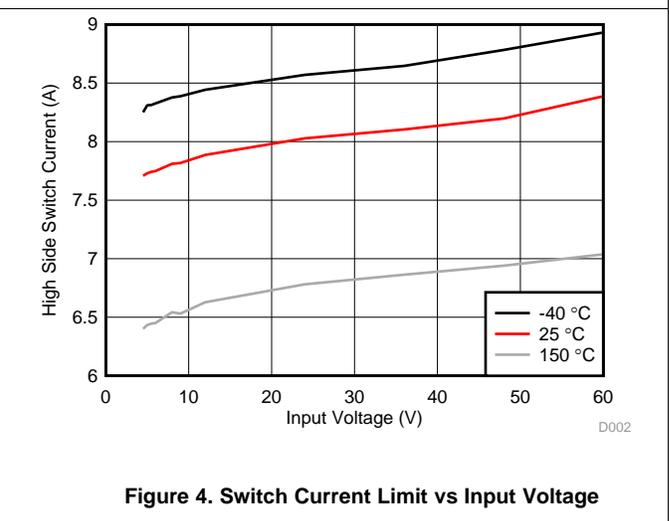
Figure 4. Switch Current Limit vs Input Voltage
