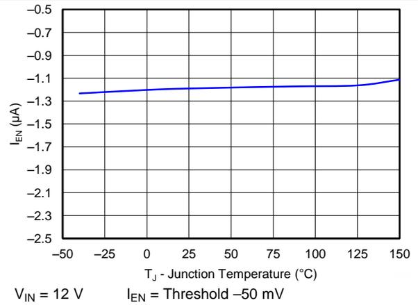
Figure 12. EN Terminal Current vs Junction Temperature
