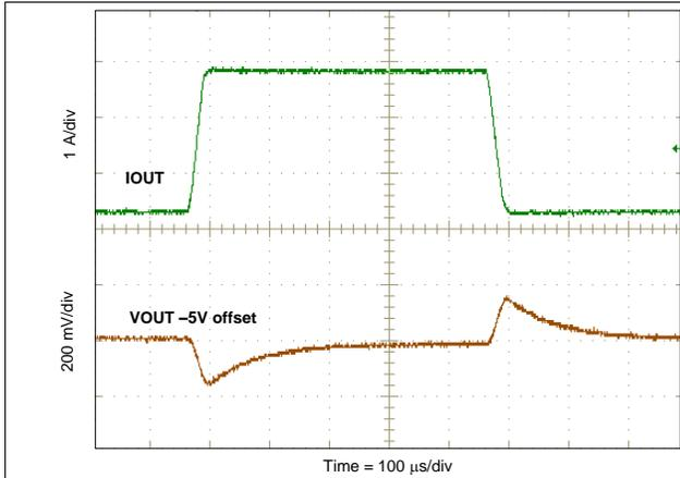
Figure 34. Load Transient
