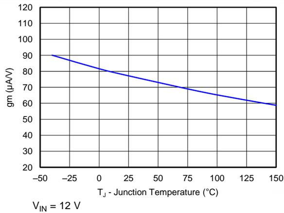
Figure 9. EA Transconductance During Soft-Start vs
