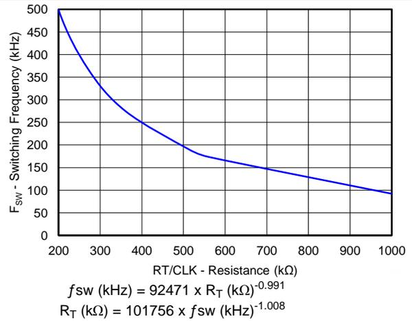
Figure 6. Switching Frequency vs RT/CLK Resistance
