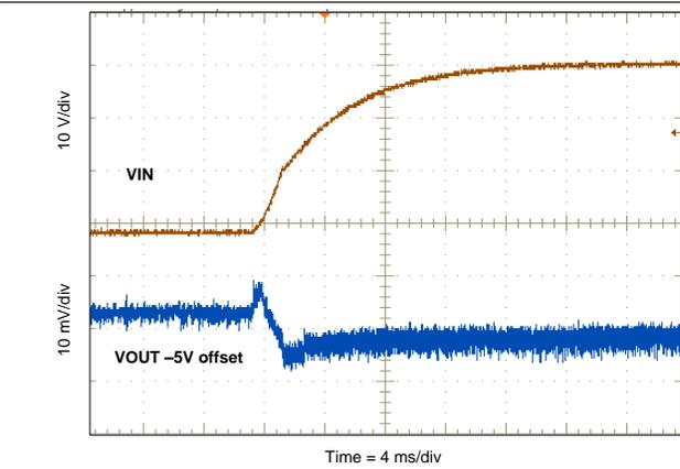
Figure 35. Line Transient (8 V to 40 V)
