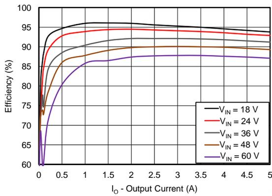
Figure 48. Efficiency vs Output Current
