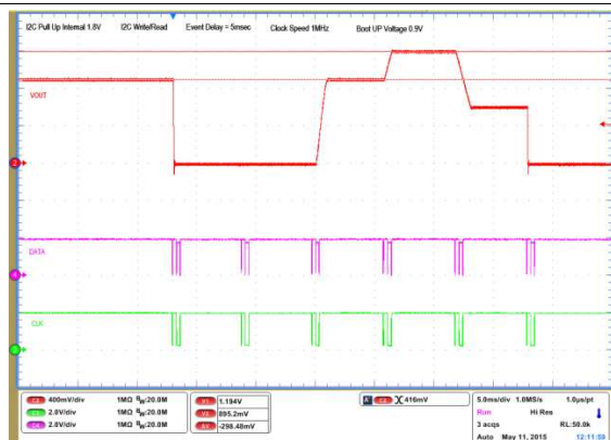
Figure 13. PMBus 1-MHz Bus Speed with 1.8-V Pullup
