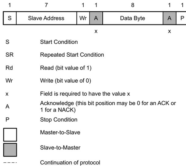
**图 8-28. I<sup>2</sup>C Read/Write Protocol Key**
