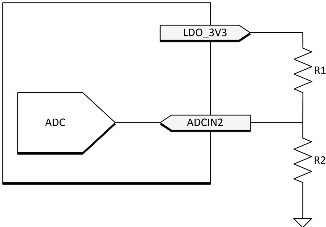
**图 8-29. I<sup>2</sup>C Address Divider**
