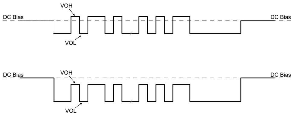
FIG 8-6. TX Driver Transmission with DC Bias
