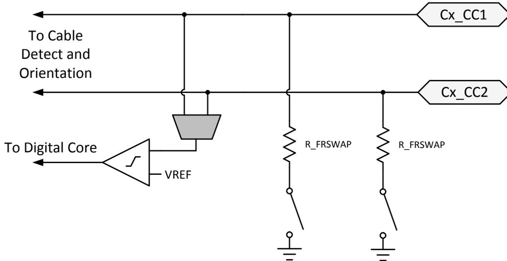
FIG 8-15. Fast Role Swap Detection and Signaling
