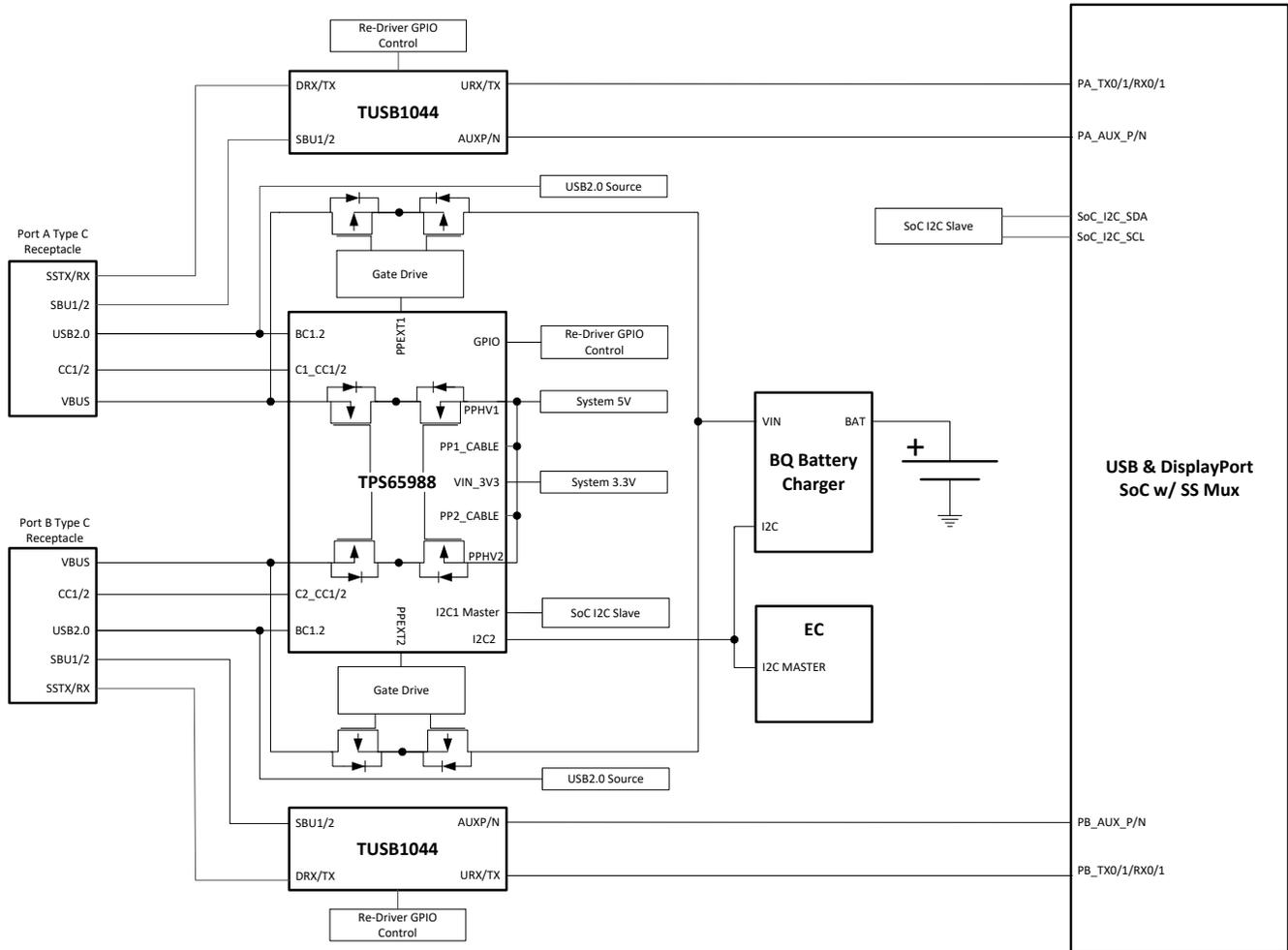
**9-9. TPS65988DJ and SoC I2C with Re-Driver GPIO**
