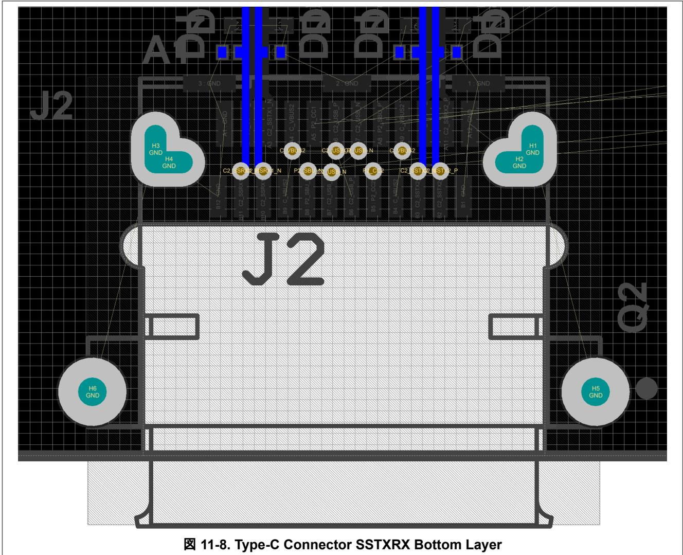
11-8. Type-C Connector SSTXRX Bottom Layer
