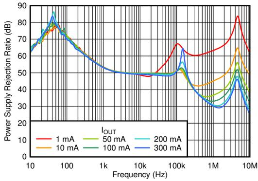
$V_{IN} = 4.3\text{ V}$ ,  $C_{IN} = 0\ \mu\text{F}$ ,  $V_{OUT} = 3.3\text{ V}$
