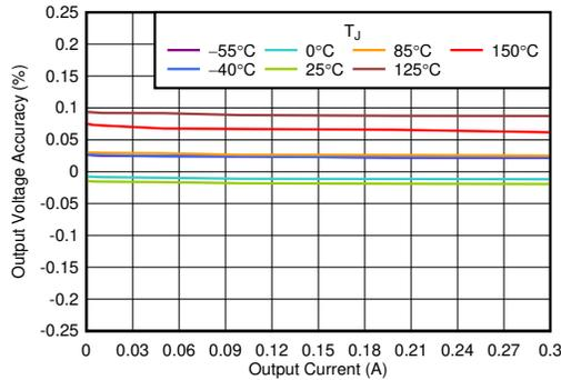
$V_{OUT} = 1.2\text{ V}$
