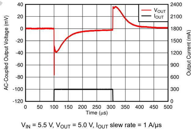
6-18.  $I_{OUT}$  Transient From  $1\text{ mA}$  to  $300\text{ mA}$
