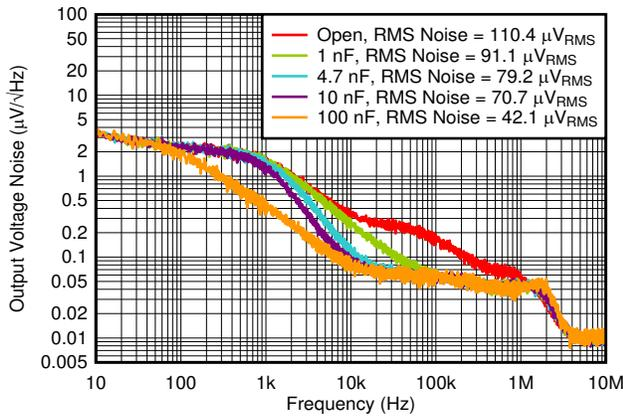
$V_{IN} = 6\text{ V}$ ,  $V_{OUT} = 5.0\text{ V}$ ,  $I_{OUT} = 300\text{ mA}$ ,
