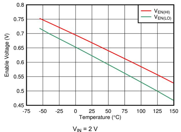
6-12.  $V_{EN(HI)}$  and  $V_{EV(LO)}$  Threshold vs Temperature
