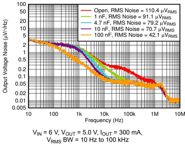
6-31. Output Noise vs Frequency and  $C_{FF}$
