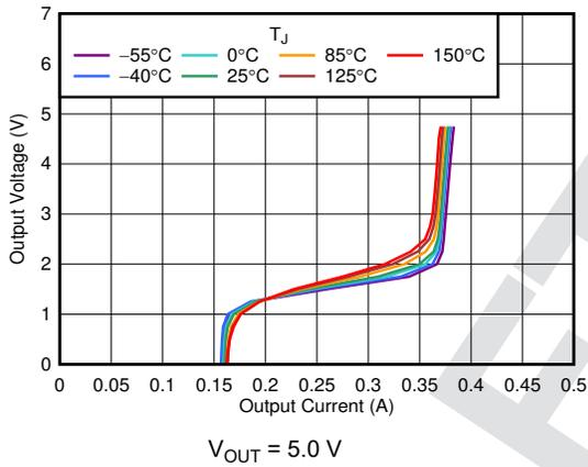
6-15. Foldback Current Limit vs  $I_{OUT}$  and Temperature
