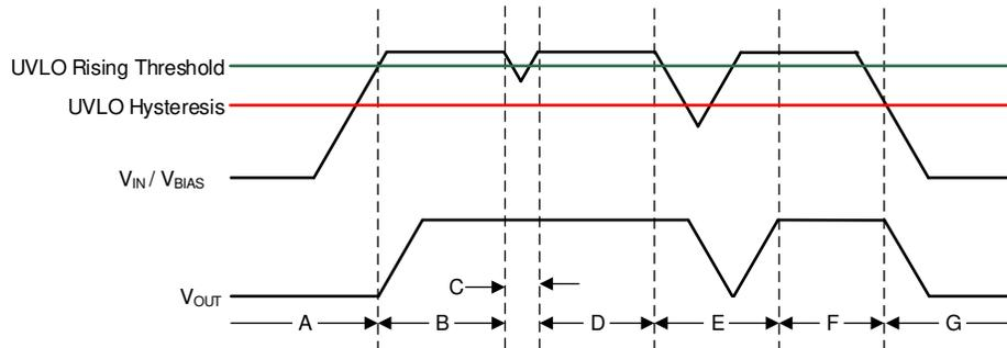
**8-2. Typical  $V_{IN}$  or  $V_{BIAS}$  UVLO Circuit Operation**
