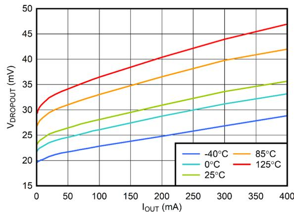
$$V_{\text{BIAS}} = V_{\text{OUT(NOM)}} + 1.4 \text{ V}, V_{\text{EN}} = V_{\text{IN}}, C_{\text{IN}} = 1 \mu\text{F}, C_{\text{OUT}} = 1 \mu\text{F}, C_{\text{BIAS}} = 0.1 \mu\text{F}$$
