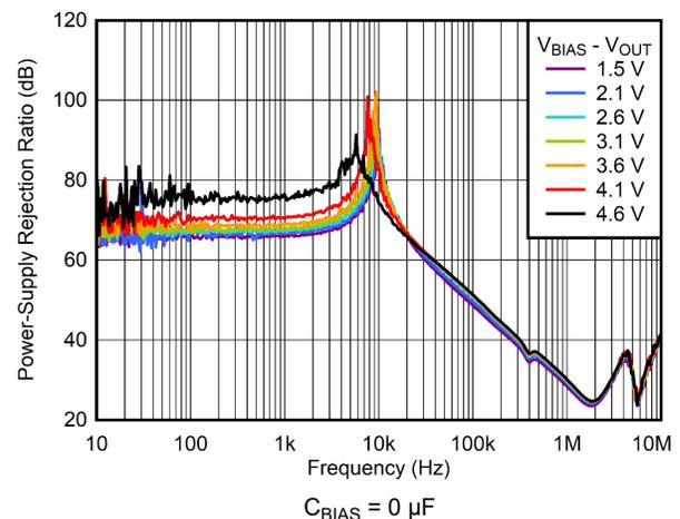
6-24.  $V_{\text{BIAS}}$  PSRR vs Frequency and  $V_{\text{BIAS}} - V_{\text{OUT}}$
