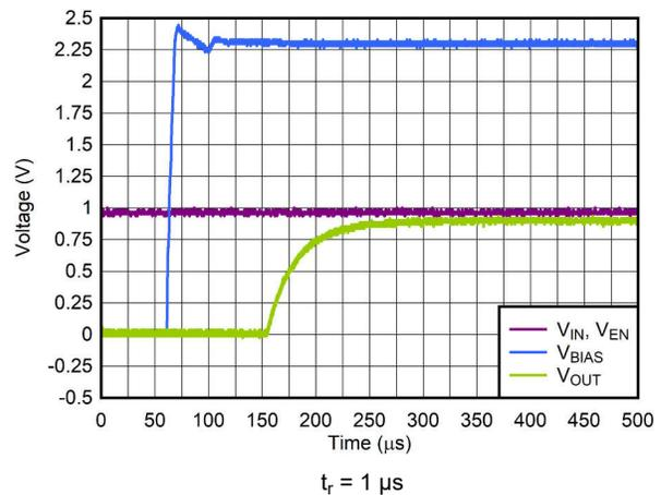
6-16. Start-Up With  $V_{\text{IN}}$  and  $V_{\text{EN}}$  Before  $V_{\text{BIAS}}$
