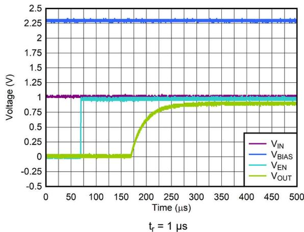
6-15. Start-Up With  $V_{\text{IN}}$  and  $V_{\text{BIAS}}$  Before  $V_{\text{EN}}$
