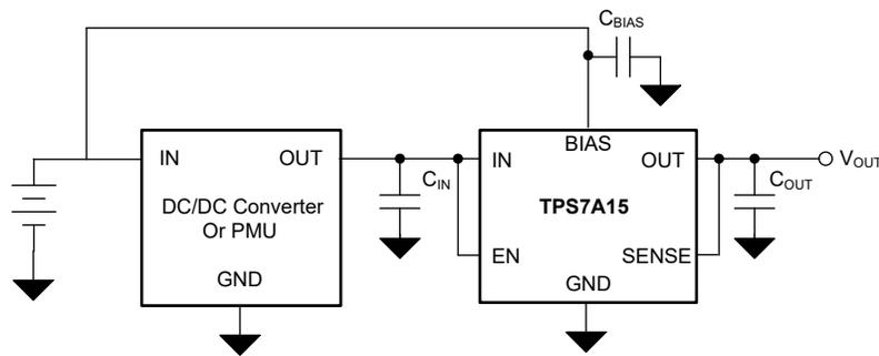
图 8-4. High-Efficiency Supply From a Rechargeable Battery
