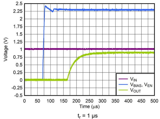
6-14. Start-Up With  $V_{\text{IN}}$  Before  $V_{\text{BIAS}}$  and  $V_{\text{EN}}$
