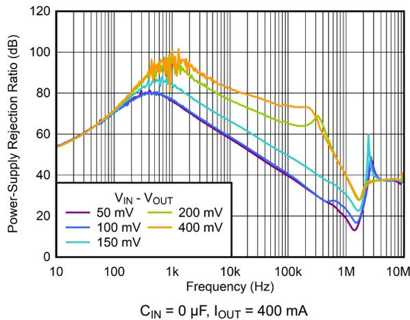
6-21.  $V_{\text{IN}}$  PSRR vs Frequency and  $V_{\text{IN}} - V_{\text{OUT}}$
