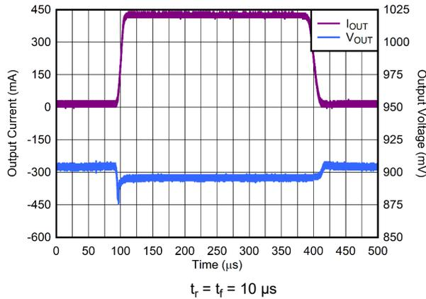
6-19. Load Transient From 100  $\mu\text{A}$  to 400 mA
