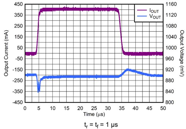
6-20. Load Transient From 100  $\mu\text{A}$  to 400 mA
