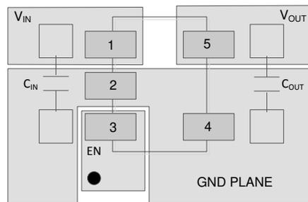
● Represents via used for application specific connections
