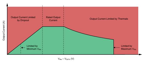
Figure 55. Continuous Operation Slope Region Description
