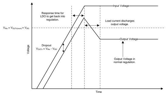
Figure 53. Start-Up Into Dropout
