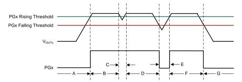
Figure 47. Typical PGx Operation
