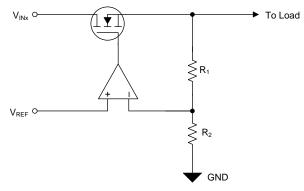
NOTE:  $V_{OUTx} = V_{REF} \times (1 + R_{1x} / R_{2x})$ .
