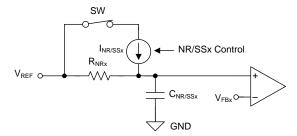
Figure 42. Simplified Soft-Start Circuit
