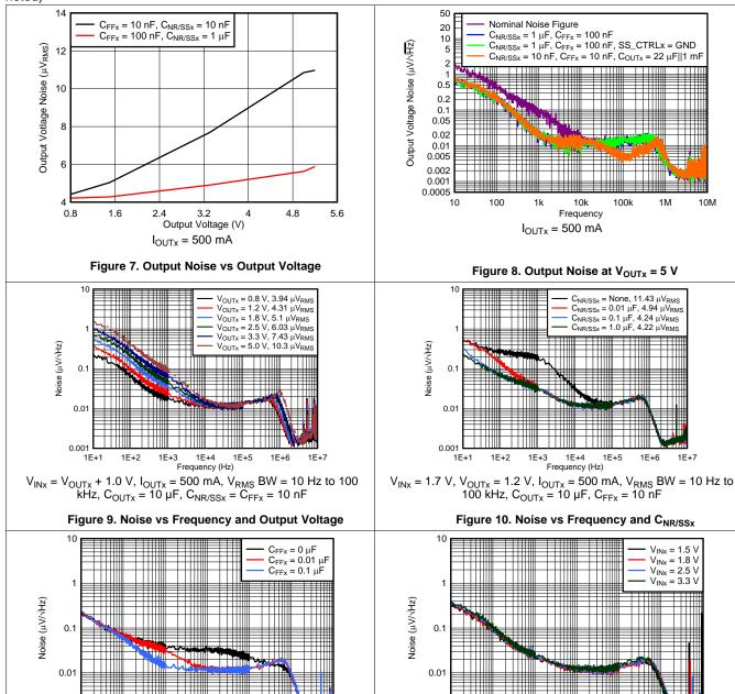
$V_{INx} = 3.8 \ V, \ V_{OUTx} = 3.3 \ V, \ I_{OUTx} = 500 \ mA, \ V_{RMS} \ BW = 10 \ Hz \ to$ 100 kHz,  $C_{OUTx} = 10 \mu F$ ,  $C_{NR/SSx} = 10 nF$
