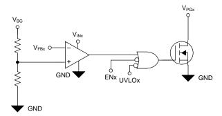
Figure 44. Simplified PGx Circuit
