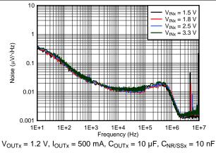
Figure 12. Noise vs Frequency and V<sub>INx</sub>
