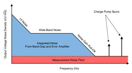
Figure 49. Output Voltage Noise Diagram
