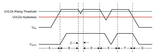
Figure 46. Typical UVLOx Operation
