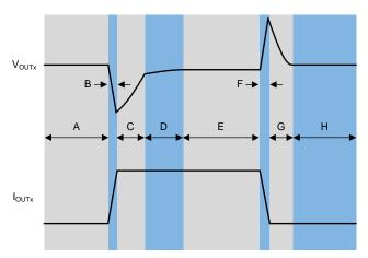
Figure 50. Load Transient Waveform
