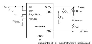
Figure 62. Application Example (Single Channel)
