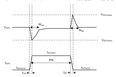
Figure 51. Simplified Load Transient Waveform
