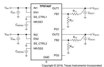
Figure 45. Adjustable Operation
