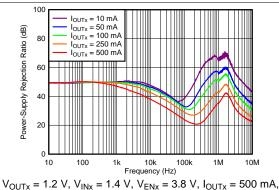
Figure 3. Power-Supply Rejection Ratio vs Frequency and Input Voltage
