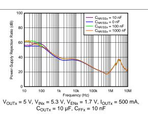
Figure 2. Power-Supply Rejection Ratio vs Frequency and C<sub>NR/SSx</sub>
