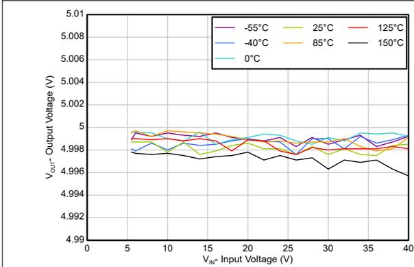
$V_{OUT} = 5V$ ,  $I_{OUT} = 150mA$
