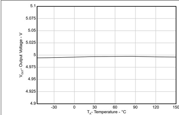
$V_{IN} = 6V$ ,  $V_{OUT} = 5V$ ,  $I_{OUT} = 150mA$
