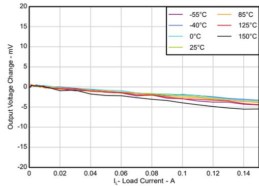
$V_{IN} = 6V$ ,  $V_{OUT} = 5V$
