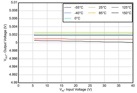
$V_{OUT} = 5V$ ,  $I_{OUT} = 100\mu A$
