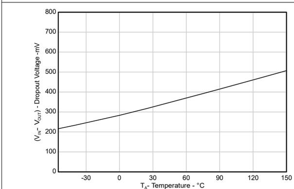
$V_{IN} = 4.9V$ ,  $I_{OUT} = 150mA$
