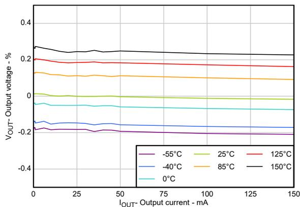
$$V_{IN} = 4.8\text{V}, V_{OUT} = 3.3\text{V}$$
