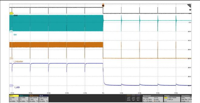
Black: DIM<sub>PWM</sub>, Light Blue: SW, Orange: Inductor Current, Deep Blue: LED Current
