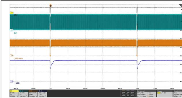
Black: DIM<sub>PWM</sub>, Light Blue: SW, Orange: Inductor Current, Deep Blue: LED Current
