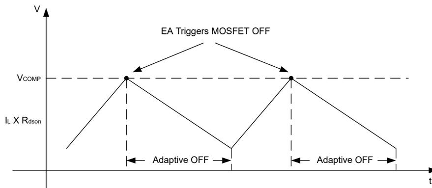
図 7-1. Adaptive off-time current mode control method
