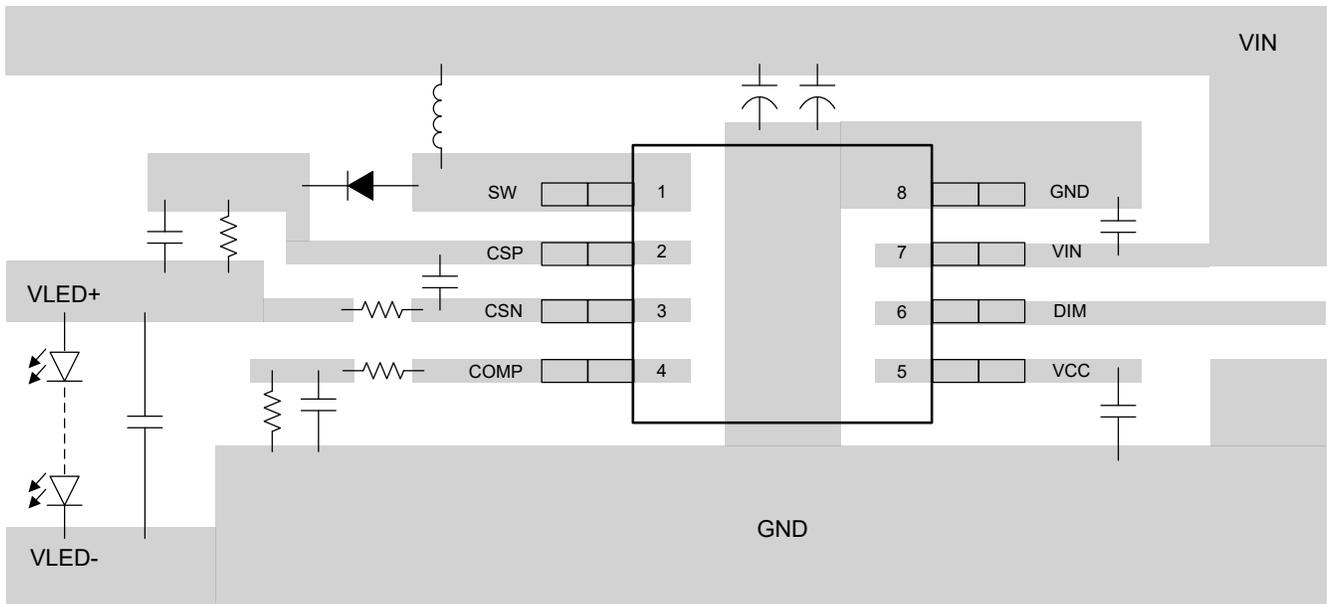
図 8-23. 8-Pin SOT583 Top View Layout Example
