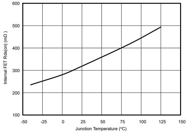
図 6-8. Switching FET Rdson vs. Junction Temperature
