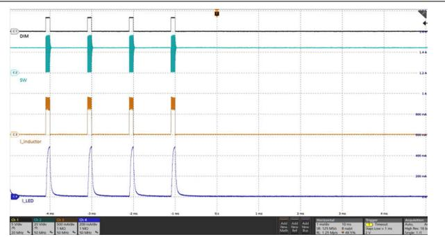
Black: DIM<sub>PWM</sub>, Light Blue: SW, Orange: Inductor Current,
