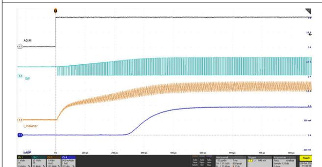
Black: DIM<sub>Analog</sub>, Light Blue: SW, Orange: Inductor Current, Deep Blue: LED Current
