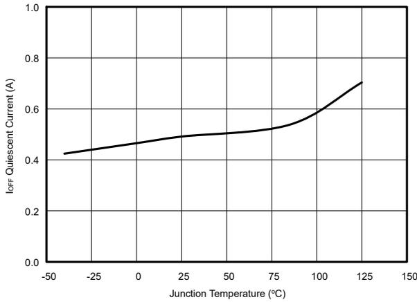
図 6-7. VIN Quiescent Current vs. Junction Temperature
