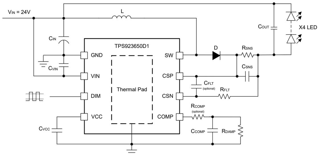
8-12. Buck-Boost, 24V Input, 0.5A Output, 4-piece WLED, PWM Dimming Reference Design
