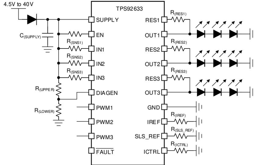
\*: 10nF ceramic capacitor is recommended for each OUTx to GND
