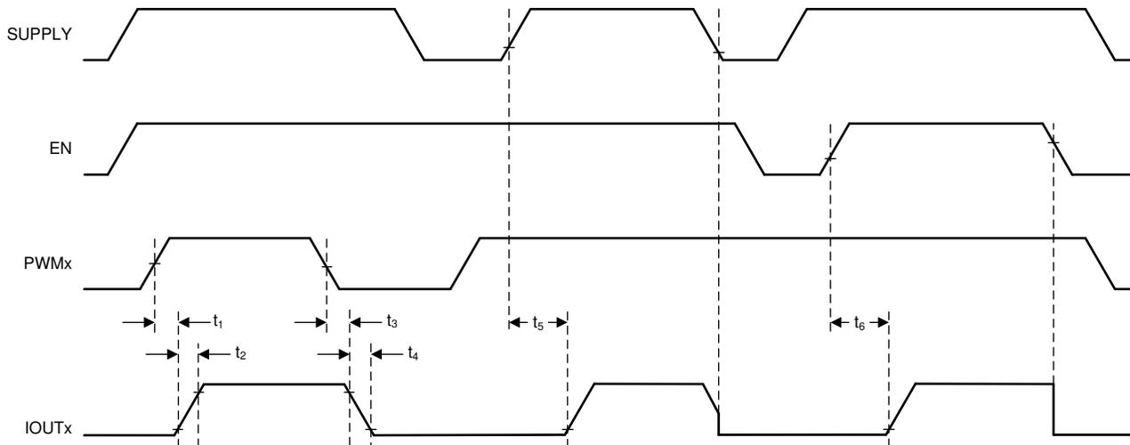
**图 7-5. Power On Sequency and PWM Dimming Timing**
