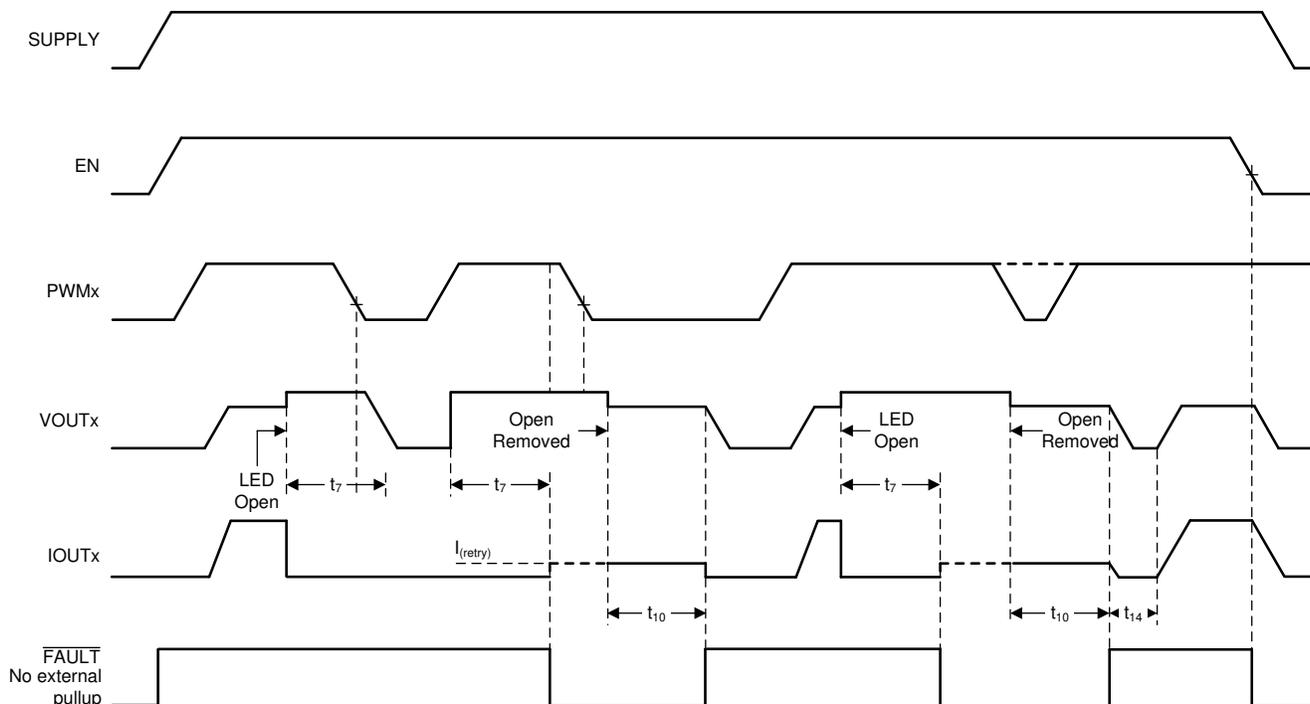
**7-8. LED Open-Circuit Detection and Recovery Timing Diagram**
