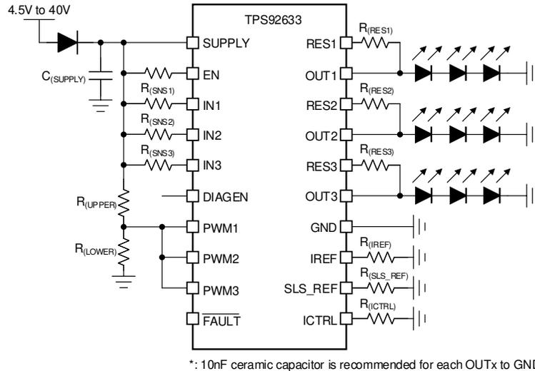
Fig 7-6. Application Schematic for Supply Control LED Brightness
