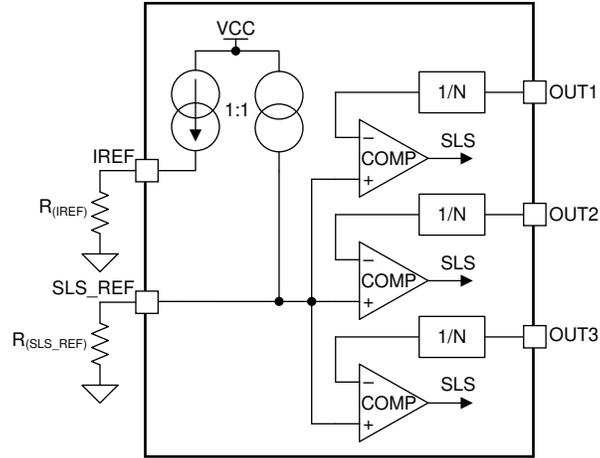
**7-9. Single LED Short-Circuit Detection Block Diagram**
