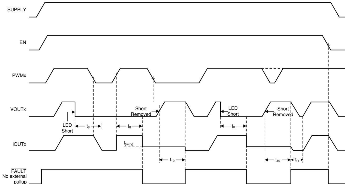
**Figure 7-7. LED Short-to-GND Detection and Recovery Timing Diagram**
