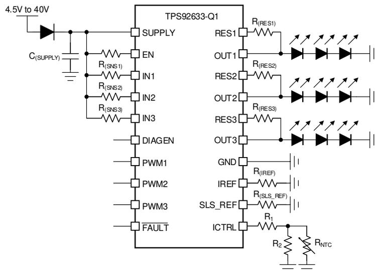
\*: 10nF ceramic capacitor is recommended for each OUTx to GND
