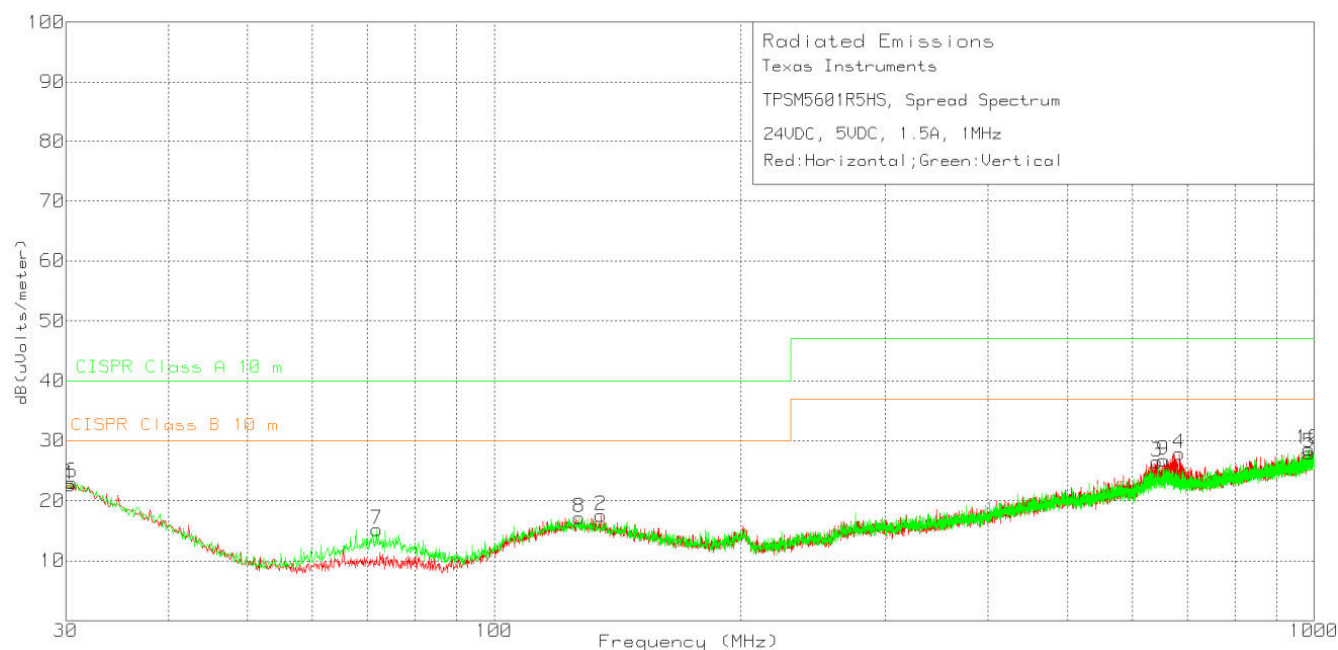
Figure 11-7. Radiated Emissions 24-V Input, 5-V Output, 1.5-A Load (Spread spectrum)
