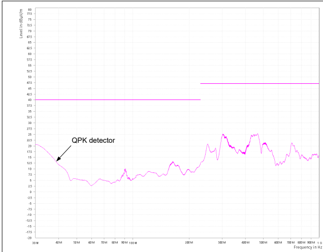
9-8. CISPR 32 Class B Radiated Emissions: Horizontal Polarization
